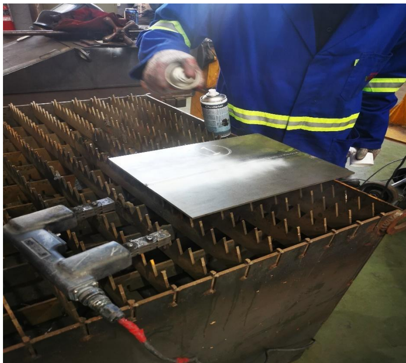
Figure 3-5: Photograph of magnetic particle testing of welded plate
