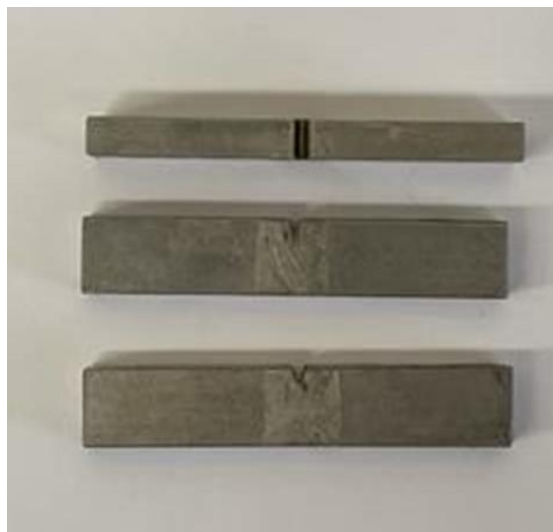
Figure 3-7: Sample of machined Charpy Impact test pieces.
