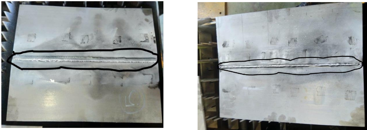
Figure 4-4: Encircled weld area after MT testing showing weld cap (left) and root run (right) of Sample 5.
