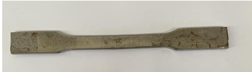
Figure 3-9: Sample of machined tensile test pieces.
