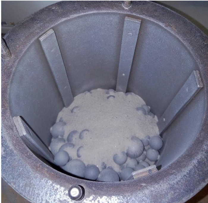
Figure 3.4: 20 and 30mm balls, quartz and lifters inside the mill
