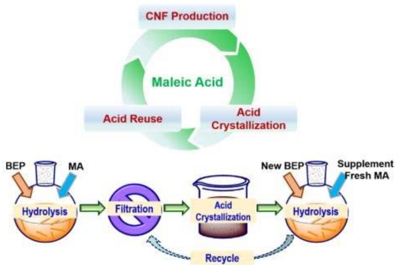
Figure 2.8: Schematic diagram for the MA hydrolysis of bleached eucalyptus pulp to produce CNFs, along with acid crystallization, acid recovery, and acid reuse (Image adapted from (Bian et al. , 2019)).
