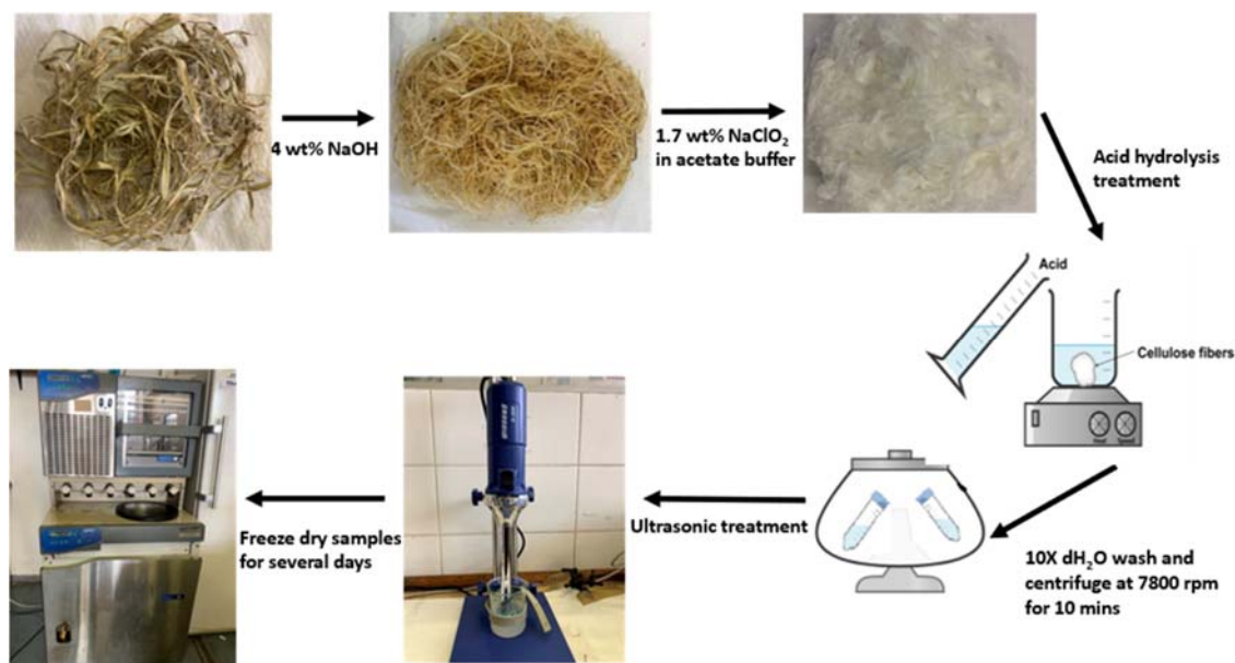
Figure 4.1: Schematic showing extraction and preparation of cellulose microfibrils from hemp bast fibres through acid hydrolysis process coupled with ultrasonic treatment.
