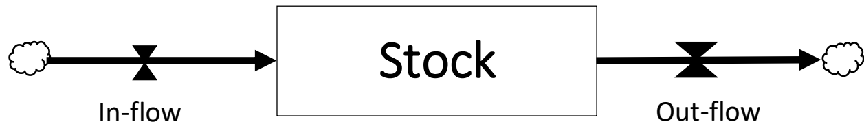
Figure 2.1 – General structure of stocks and flows in dynamic systems (Source, Sterman (2000))
