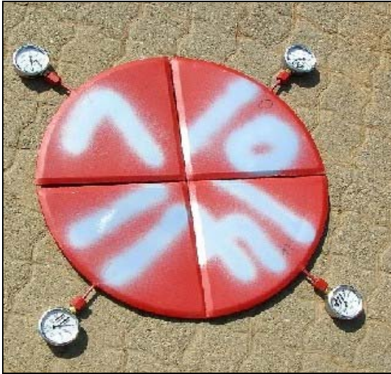
Figure 5.12 Quadrant loadcells consisting of four separate units Figure 5.13 Undergoing calibration testing
