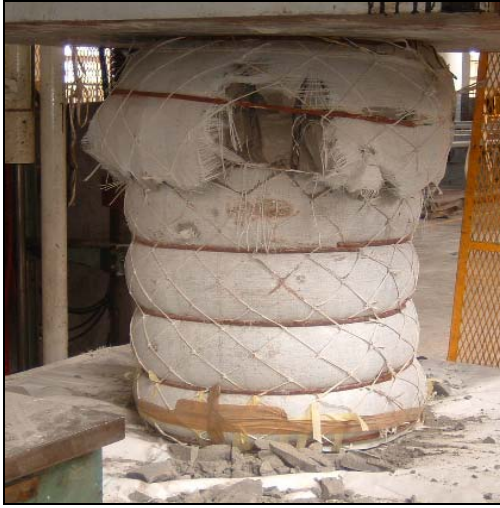
Figure 4.10 A 750 mm diameter RSS pack in the press at 150 mm compression
