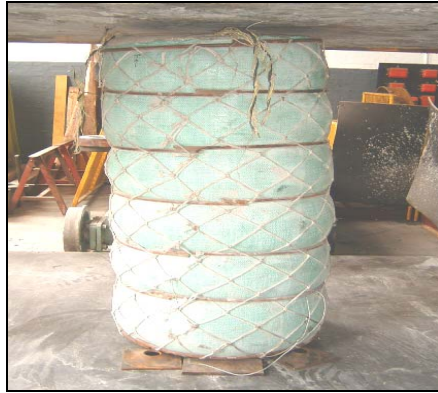
Figure 4.12 550 mm diameter RSS pack before a press test
