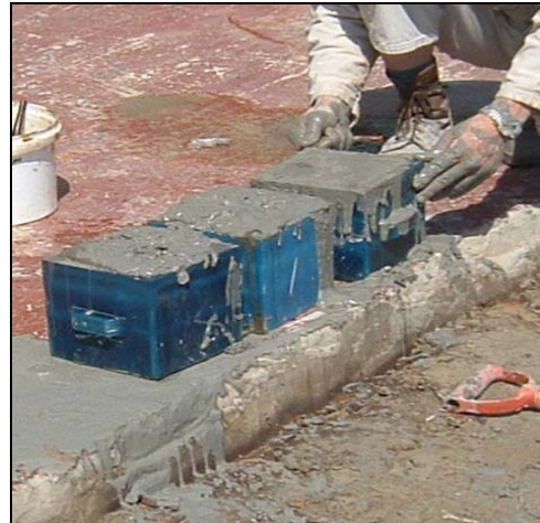
Figure 2.2 Preparation of 150 mm grout cubes
