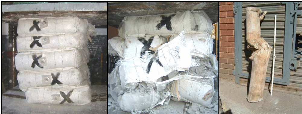
Figure 4.19 A 900 mm square Taupack at different stages of a compression test with the mine pole that was contained within
