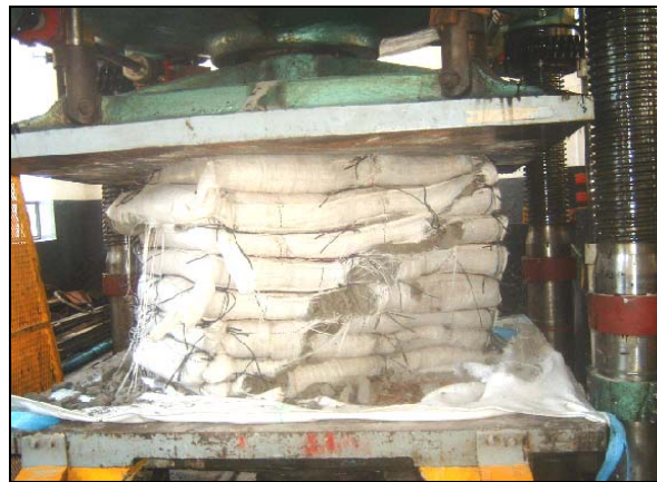
Figure 4.27 A Cempack being press tested
