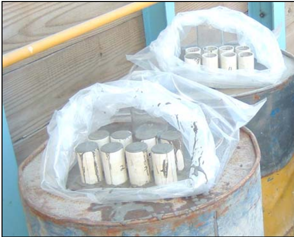
Figure 2.1 Preparation of 43/84 mm grout cylinders
