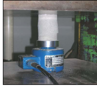
Figure 2.4 Grout cylinder first tested after one day undergoing re-testing after 56 days
