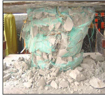
Figure 4.13 550 mm diameter RSS pack after a press test
