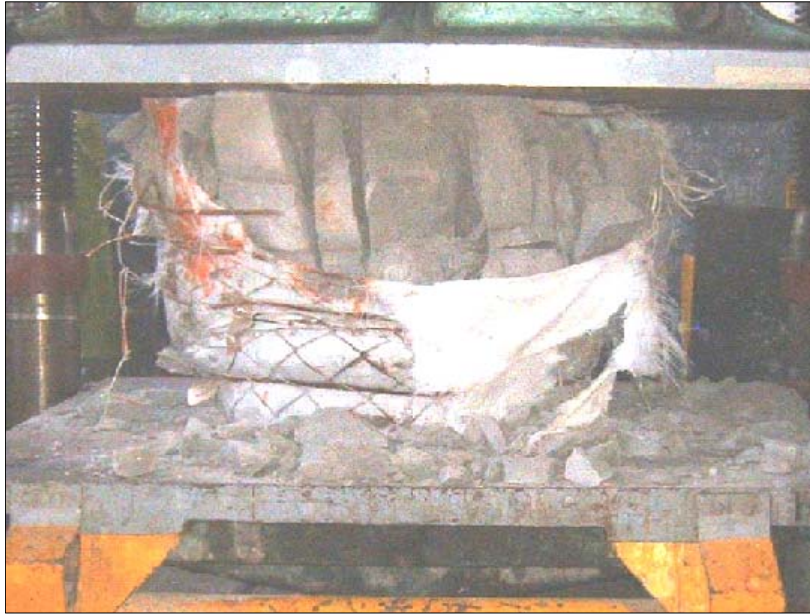
Figure 4.8 900 mm diameter pack at 36% compression
