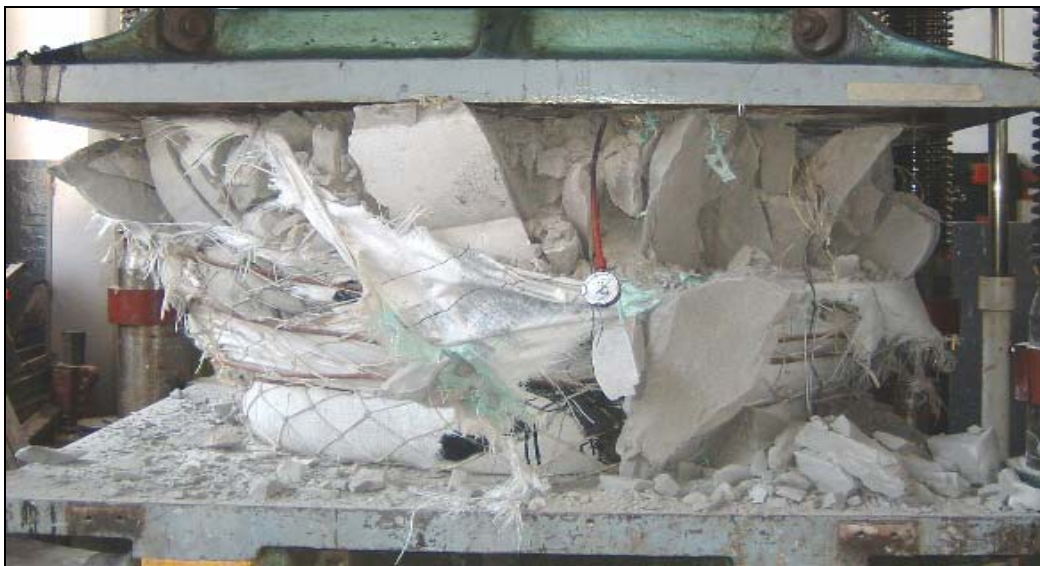
Figure 4.6 1200 mm diameter RSS pack showing lateral dilation and failure of the upper rings
