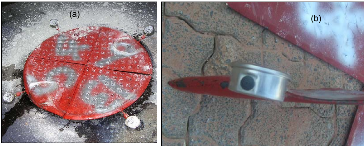
Figure 5.15 (a) Damaged loadcells after the press test (b) Side view of a damaged cell
