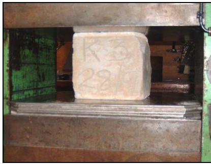
Figure 2.5 Grout cube undergoing strength testing
