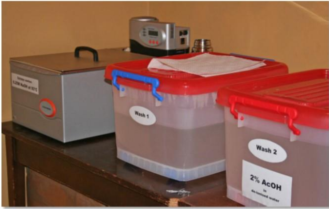
Figure 20: Laboratory apparatus used for etching and washing (From: Parc RGM).
