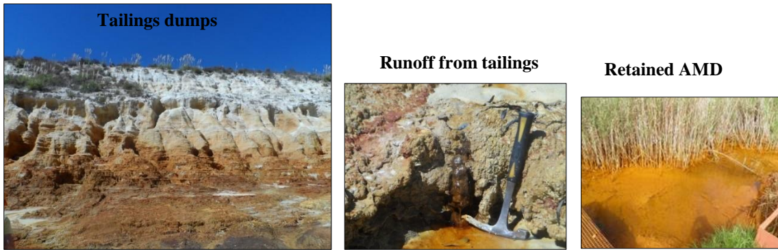
Figure 27: Observed impact of abandoned gold mine tailings on surface water samples whereby during a rainy season leachate are generated from the gold mine tailings and be transported to nearby water points whereby they become deposited.
