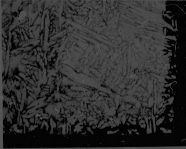
FIGURE 4.20 : SELECTIVE ATTACK ON THE \beta -PHASE IN NAVAL BRASS. EXPOSURE : 1000 h AT 150 °C (x 80)
