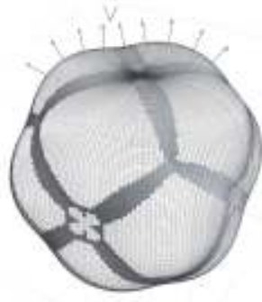
Figure. 2.4. Three dimensional ST sheet of the slowness surface for a Si crystal. Shaded regions are of saddle curvature and unshaded regions have convex or concave curvature (Calculated by A.G. Every).
