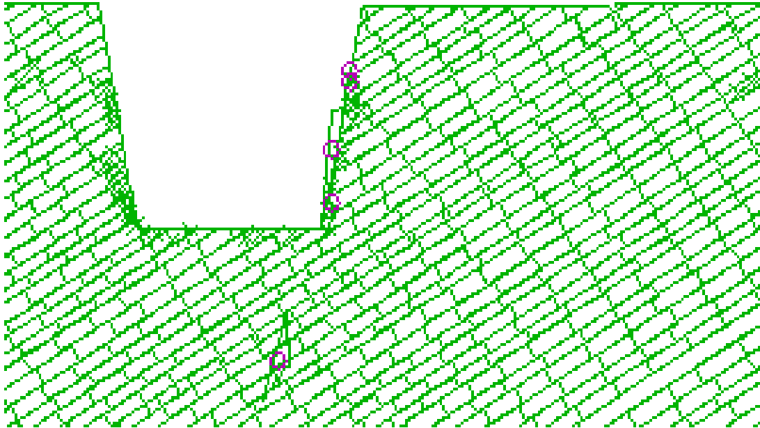
Figure 62: Standard deviations in bedding plane and joint spacings of \pm 25\% of mean spacings
