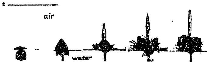
Figure 2.20 Water jet produced by accelerating a solid sphere initially immersed in liquid towards the free surface (Kedrinskii 1978)
