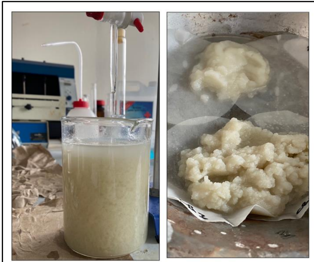
Figure 3.3: The precipitation of chitosan bentonite beads by dropping NaOH into the chitosan bentonite mixture
