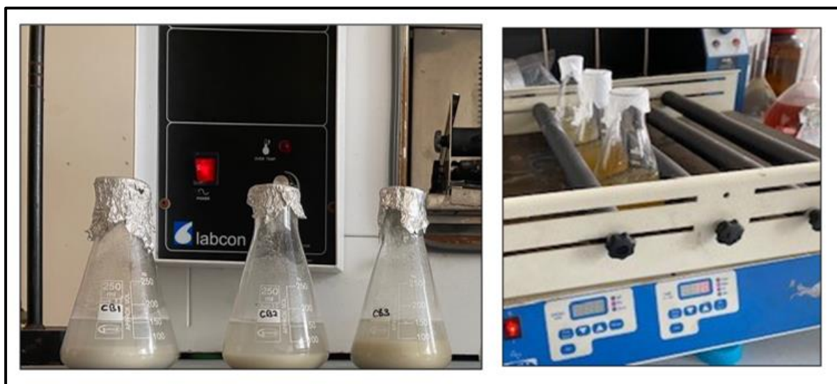
Figure 3.2: Crosslinking of chitosan and bentonite under constant stirring in a shaker
