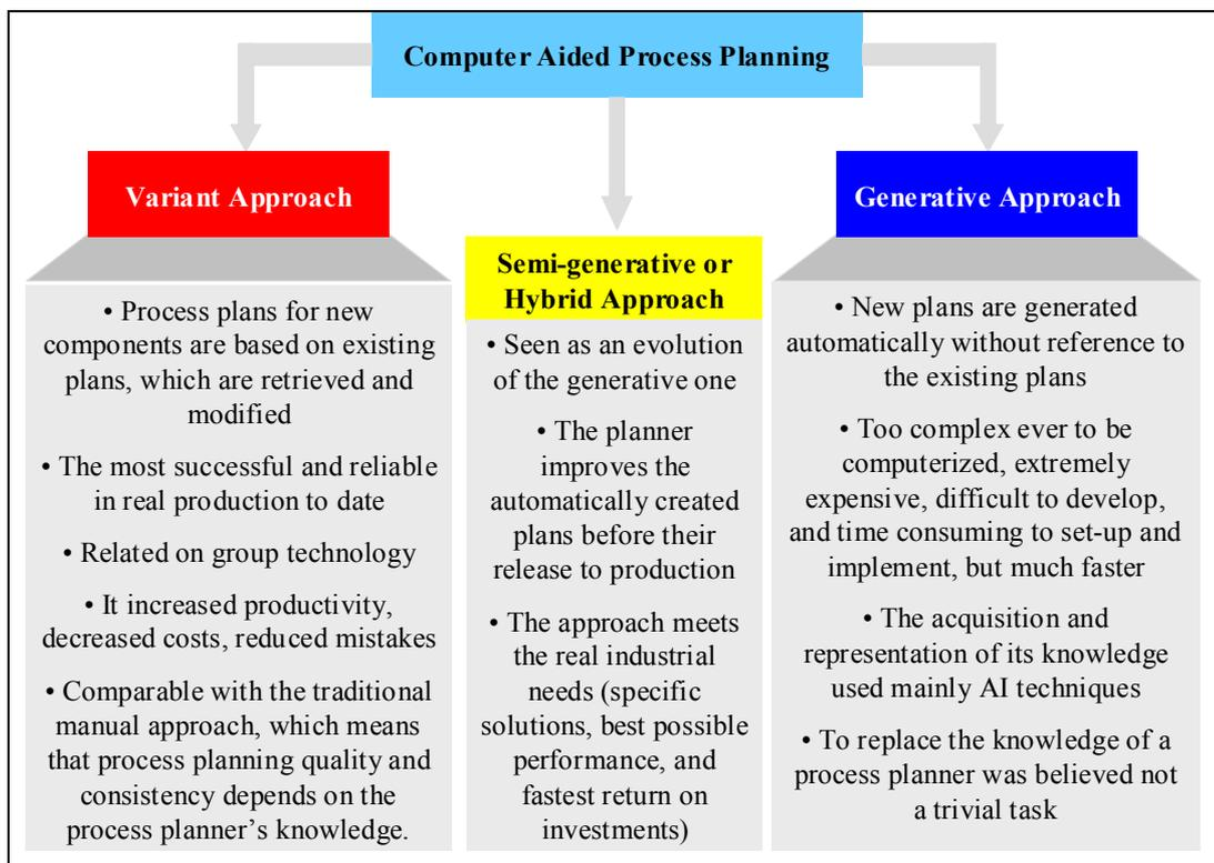
**Figure B.1** CAPP classification: The source of the process plans was the key method of CAPP systems classification (Alting and Chang 1989, Zhang 1994, Hugh 1994, Cay and Chassapis 1997, and Rozenfeld and Kerry 1999)
