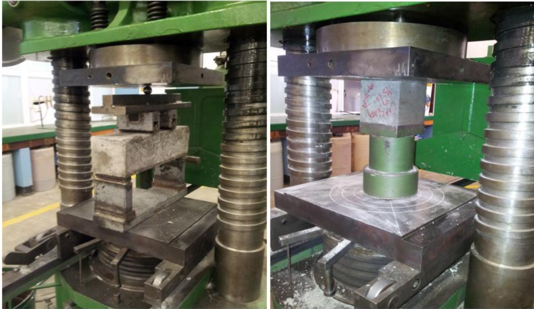
Figure 3.12(a): Flexural strength test performed on concrete prisms Figure 3.12(b): Compressive strength test performed on concrete cubes
