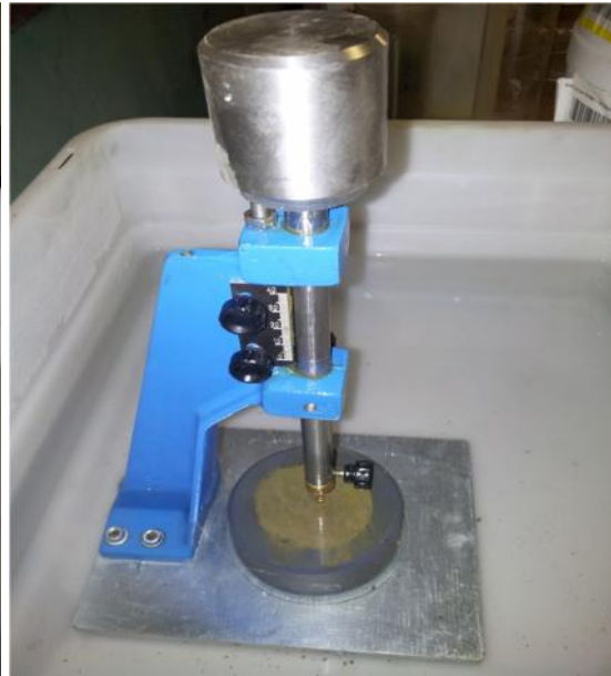
Figure 3.6: Final setting time setup
