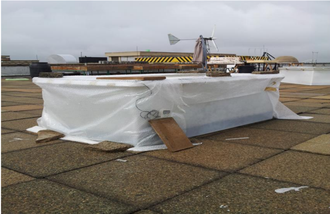
Figure 3.11 a) Concrete cubes cured inside the solar chamber
