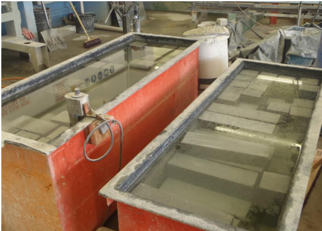
Figure 3.10: Concrete cubes and beams immersed in water curing tanks
