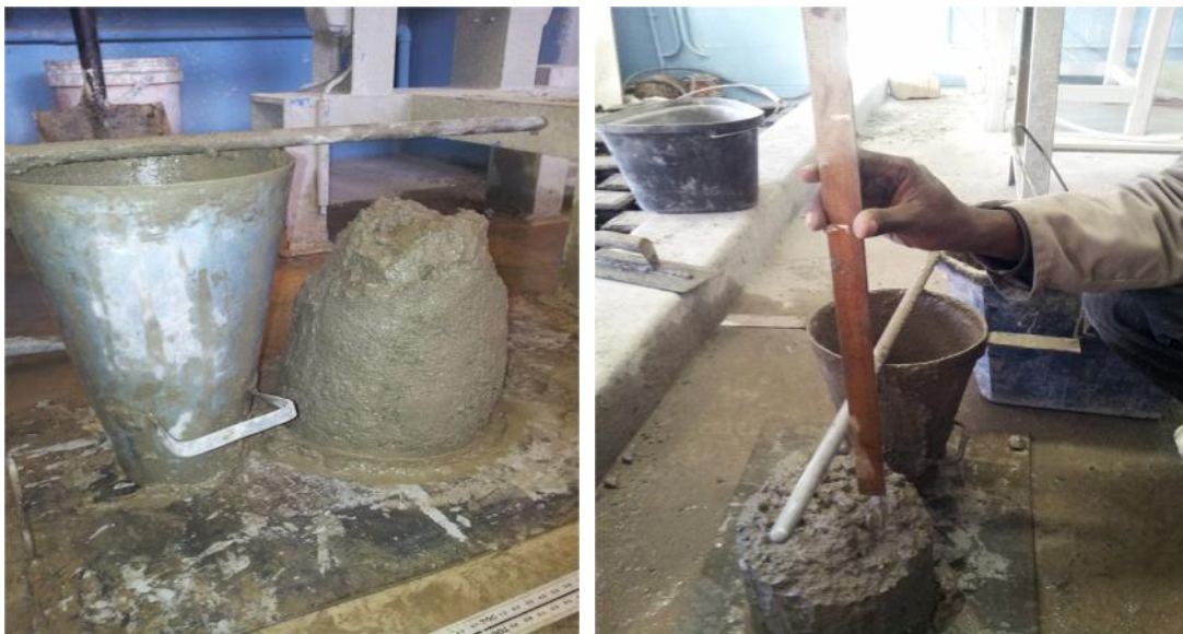
Figure 3.8: Determination of the slump of fresh concrete from the pan mixer
