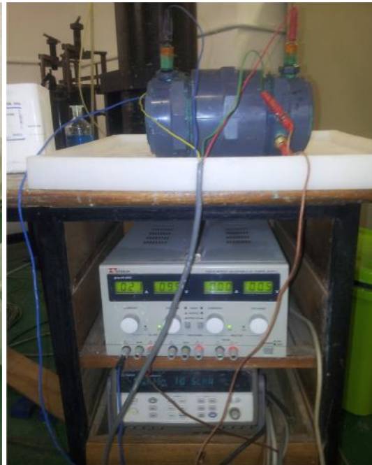
Figure 3.19: Concrete disc being tested for chloride conductivity
