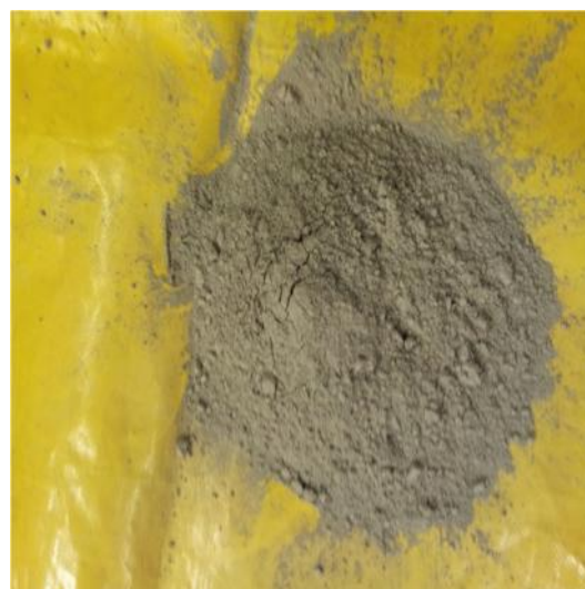
Figure 3.2: Pulverised Copper Slag
