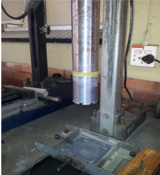
Figure 3.13: Coring drill for cutting concrete discs specimens
