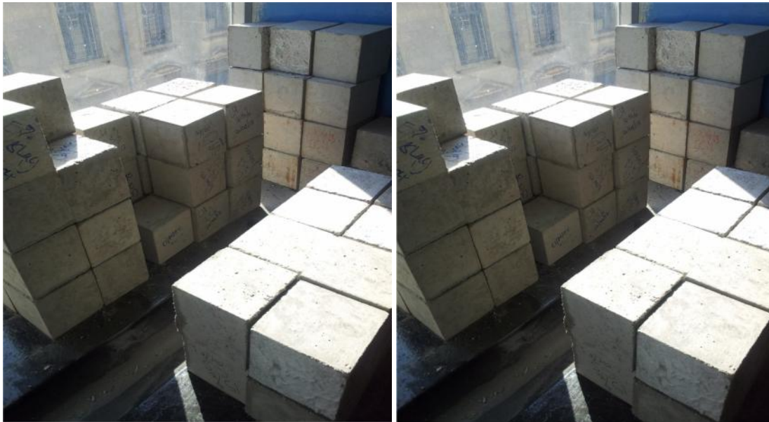
Figure 3.9: Stack of concrete cubes cured in ambient air for up to 90 days
