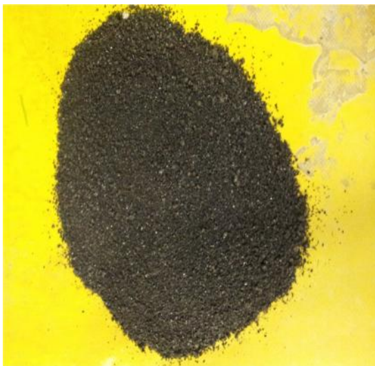
Figure 3.1: Granulated Copper Slag
