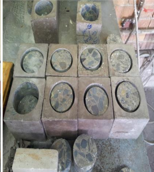
Figure 3.14: Cored discs specimens of average diameter 70 mm
