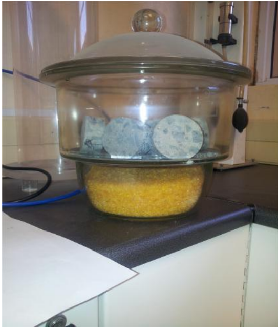
Figure 3.16: Cored concrete discs samples stored in a desiccator
