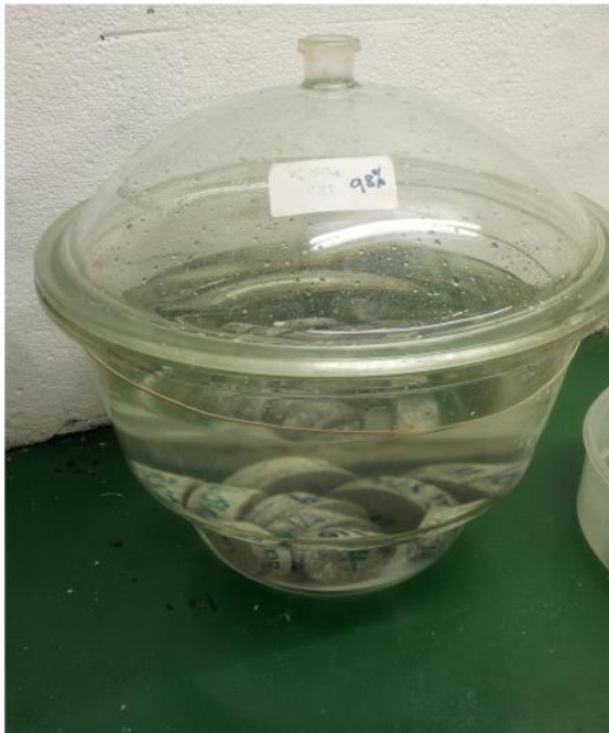
Figure 3.18: Concrete discs samples immersed in NaCl Solution
