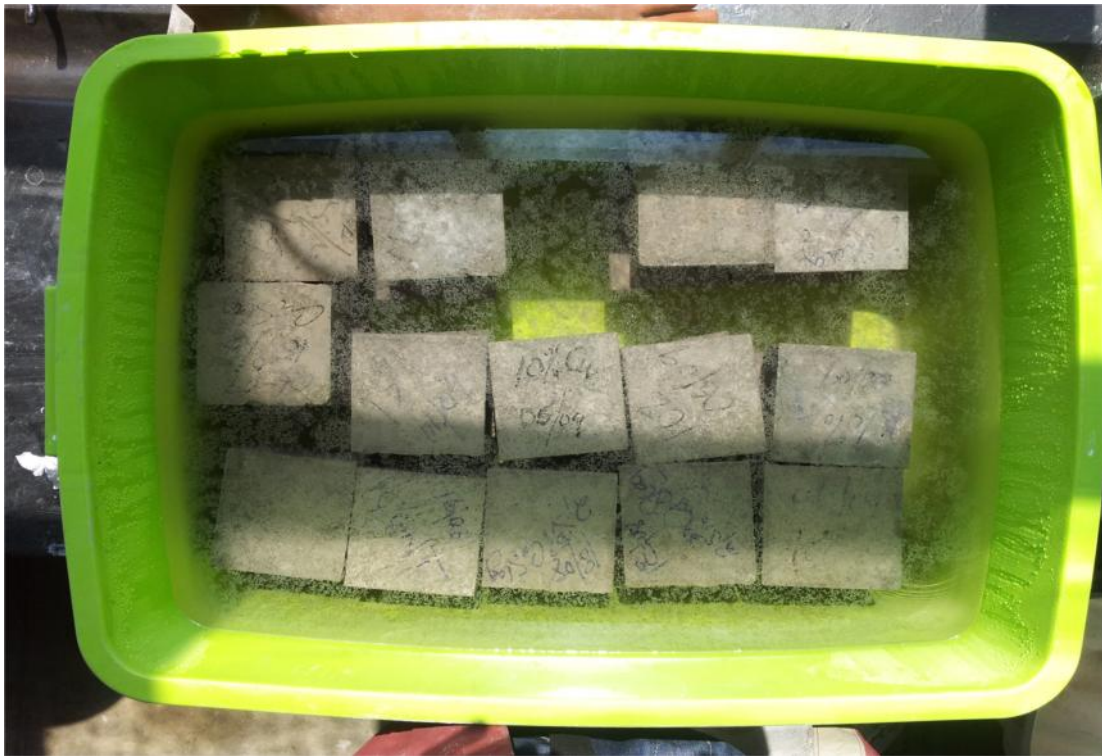
Figure 3.20: Concrete cubes immersed in 50g per litre of \text{Na}_2\text{SO}_4 solution
