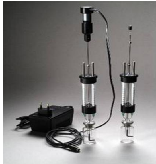
Figure 3.7 b) Electronic syringe for mixing the cement paste
