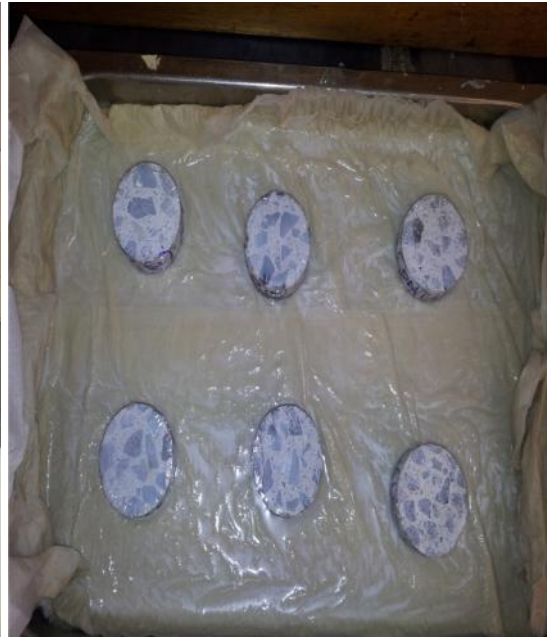
Figure 3.17: Cored concrete discs samples being tested for sorptivity
