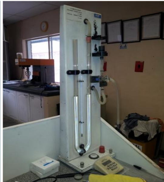
Figure 3.4: Blaine air permeability test setup
