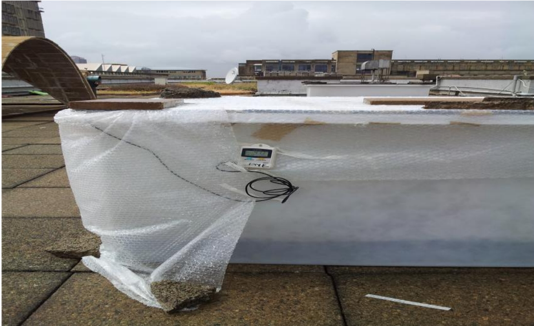
Figure 3.11 b) A temperature and humidity digital probe attached to monitor the internal conditions
