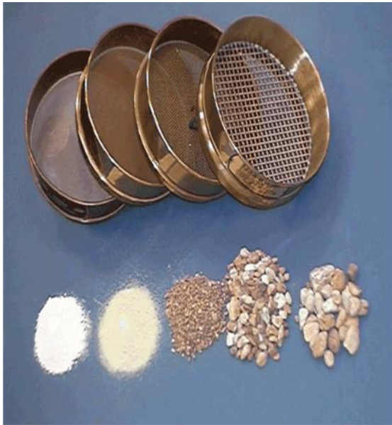
Figure 3.3: Stack of sieves for fineness test
