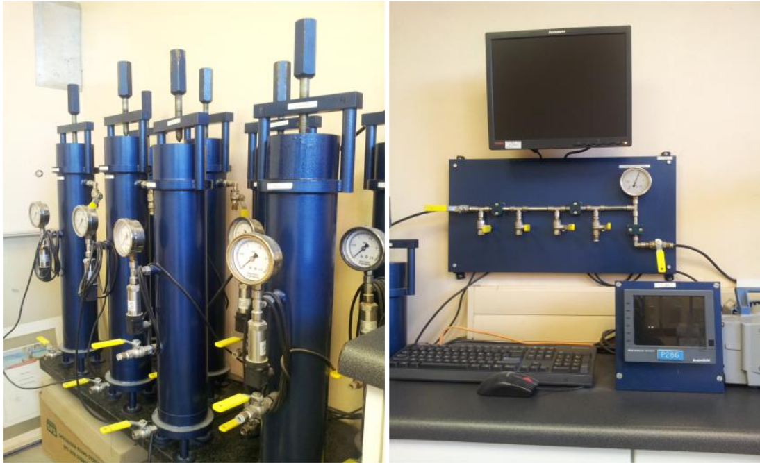
Figure 3.15(a): Oxygen permeability index measuring setup Figure 3.15(b): A computer data logger
