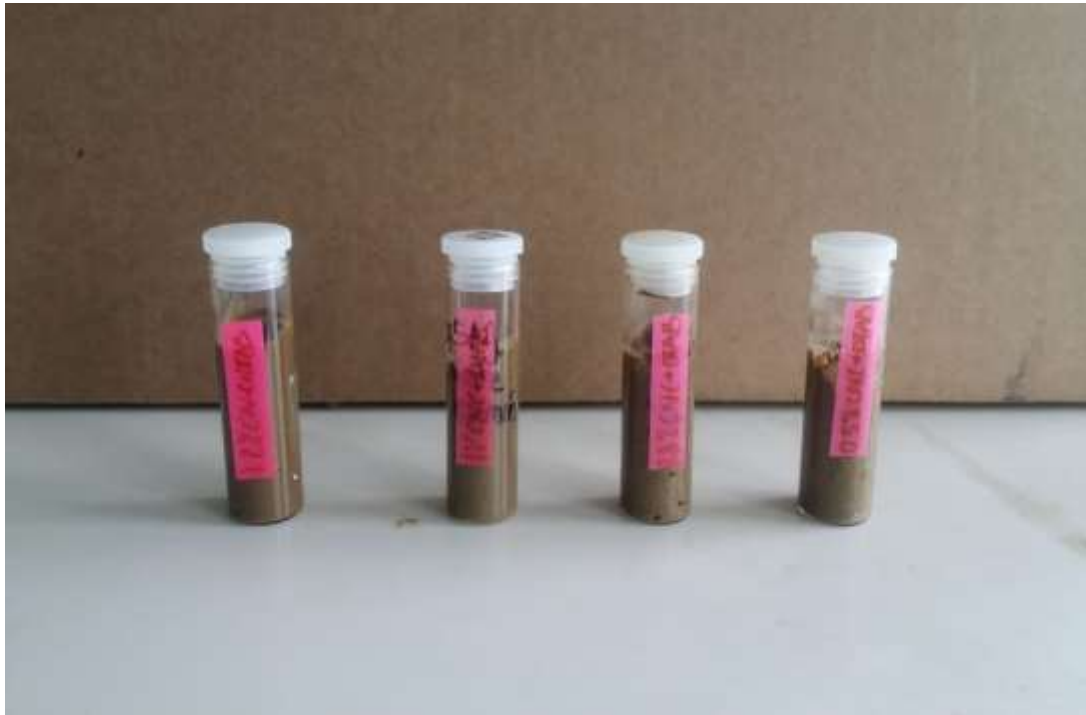
Figure 28: Emulsion prepared with DTAB as surfactant and crude oil
