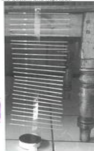
Figure 1 The wave model you are making. The tape must be held at the bottom and kept taut.
