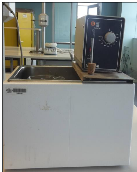
Figure 3.1. Water bath with thermometer and Controller
