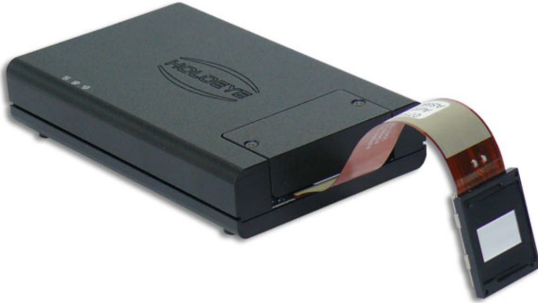
FIGURE 2.1: A representation of a Pluto-2.1 Holoeye LCoS-SLM with a full HD resolution ( 1920 \times 1080 ) where each pixel has a pitch of 8 \mu m . The device is made up of three components, a control electronic board, a flex cable and a LCD [107]
