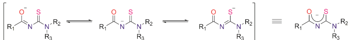
Scheme 1: Resonance structures showing possible negative charge distribution on oxygen, nitrogen, and sulfur in the anionic disubstituted acylthiourea ligand.
