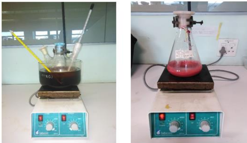
Figure 3-2: Desilication of the zeolite support (left) and preparation of the Co/H-ZSM-5 catalyst via IWI using the desilicated zeolite
