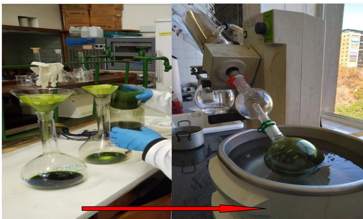
Figure 3-5: Picture showing the filtration of MLE (left) and evaporation of alcohol during the extraction process of MLE in the laboratory
