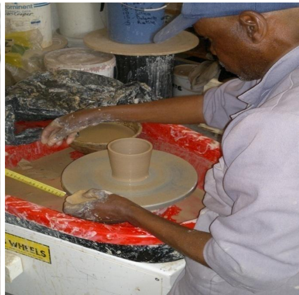
Figure 2 Wheel-working (throwing) technique
