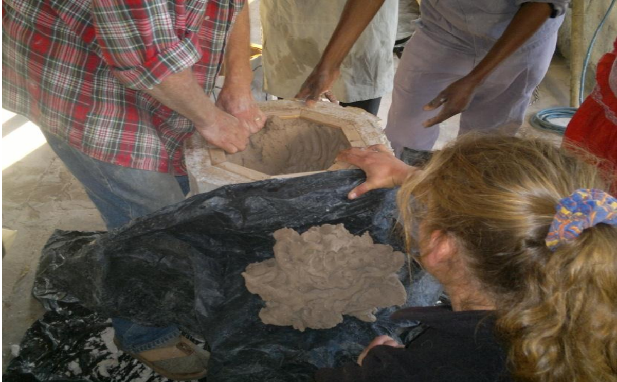
Figure 5 Creating a mould using a slabbed prototype (sources from the NWCDI master crafter training report 2012)
