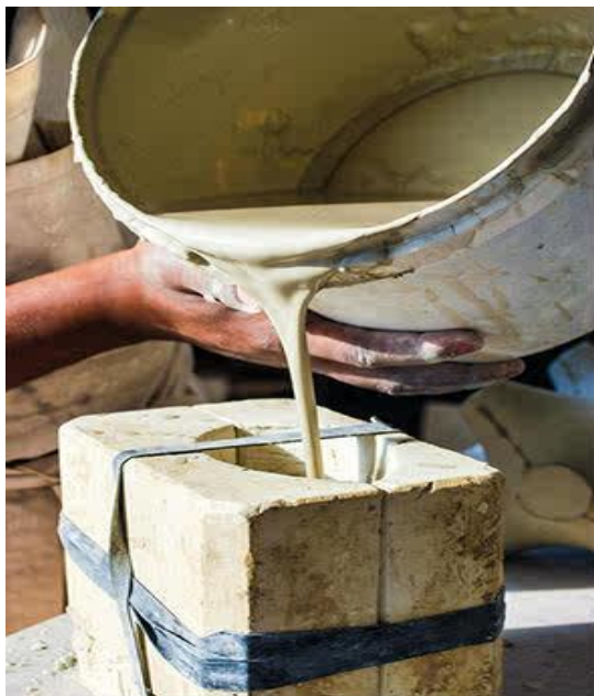
Figure 3 Pouring slip into a two piece plaster mould (sourced from the Imiso Ceramic website)
