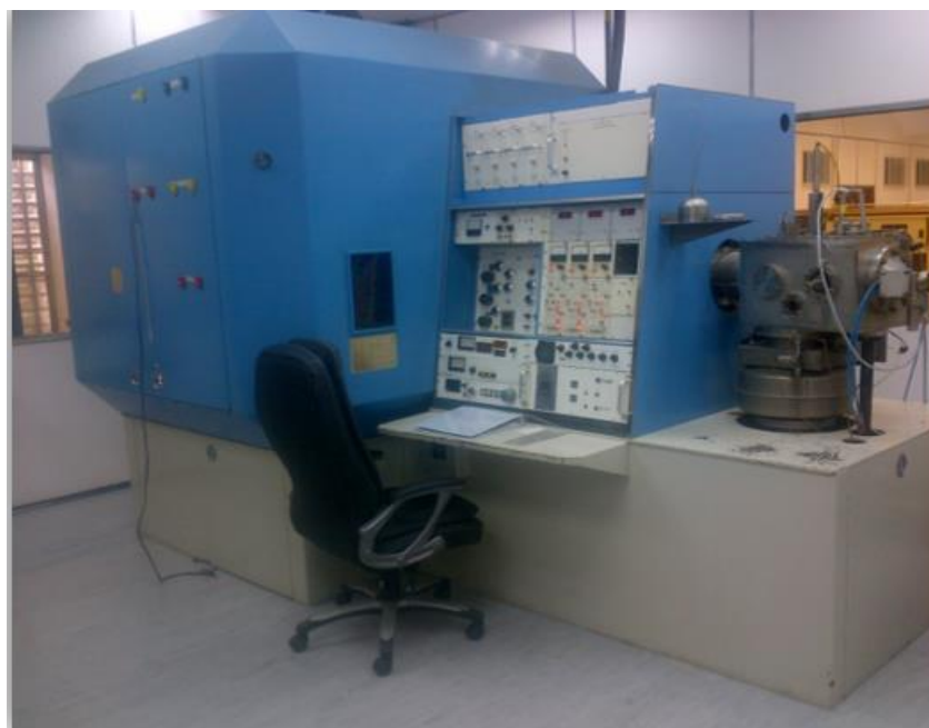
Figure 4.9: The Varian-Extrion 200-20A2F Ion implanter located at iThemba LABS (Gauteng), South Africa.
