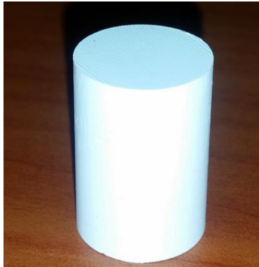
Figure 4.5: Hot pressed polycrystalline hexagonal boron nitride (h-BN) sample in the form of a rod.
