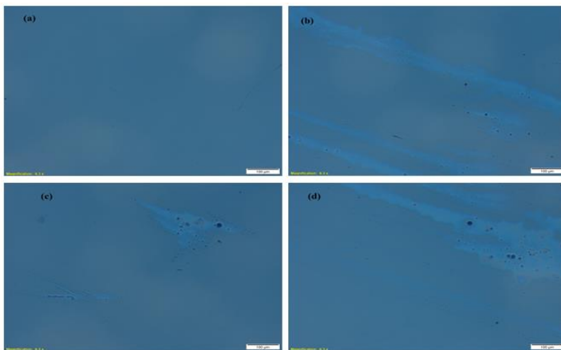
Figure 23: Asphaltene aggregation stages in oil + 10% of I.A. + n-C 7 sample. (a) 0mL added n-C 7 - 0min; (b) 2ml added n-C 7 - 542min; (c) 6.1ml added n-C 7 - 631min; (d) 8.5mL added n-C 7 - 720min.
