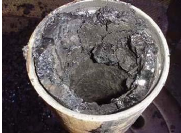
Figure 7: Asphaltene oil deposition problem. (Eigner, 2016).
