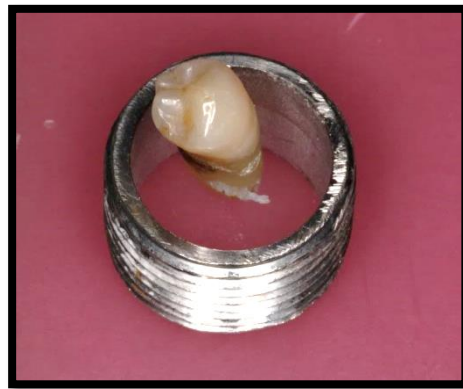
Figure 3.1 Stainless steel rings (Bencore) of 1.5cm by 1.2cm on a pink baseplate wax
