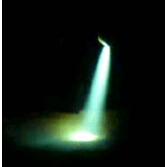
Figure 4.3 4 kA arc in air, struck on a graphite block
