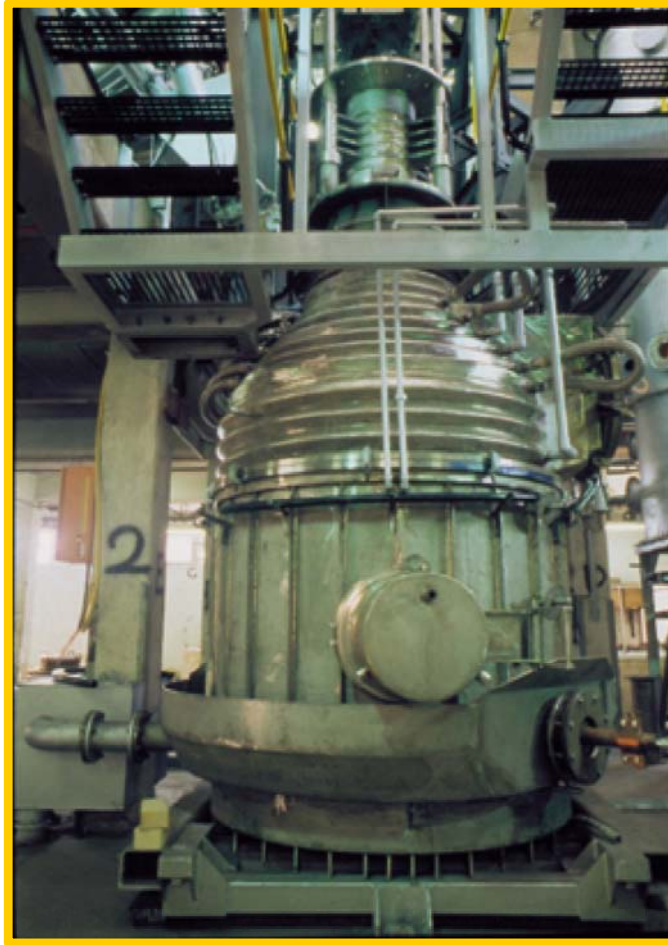
Figure 2.28 DC arc furnace for magnesium production
