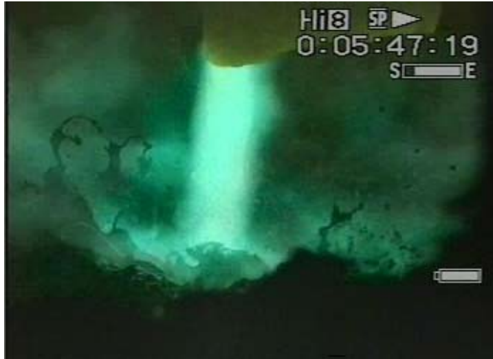
Figure 4.28 Thicker arc with splashing at 8.1 kA
