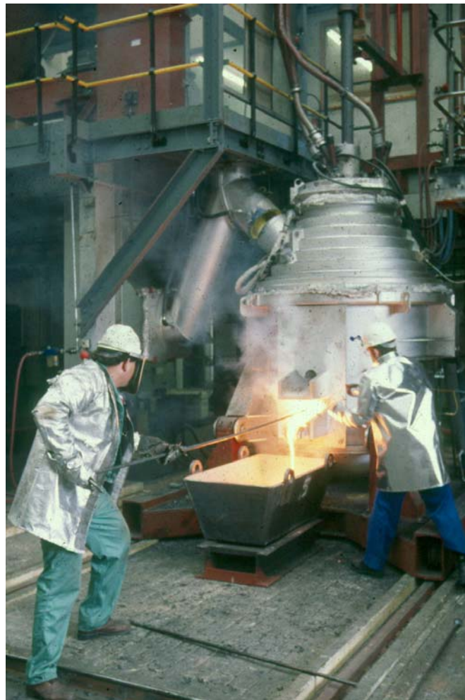
Figure 2.8 Mintek's 1 t/h (3.2 MVA) DC arc furnace pilot plant, 1984
