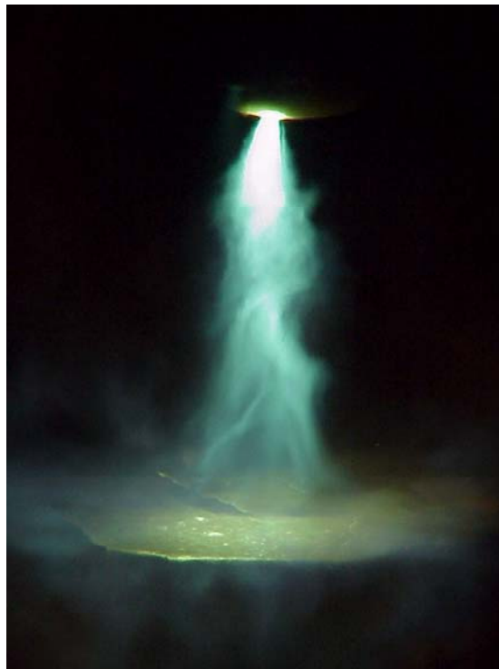
Figure 4.24 Arc about to become unstable
