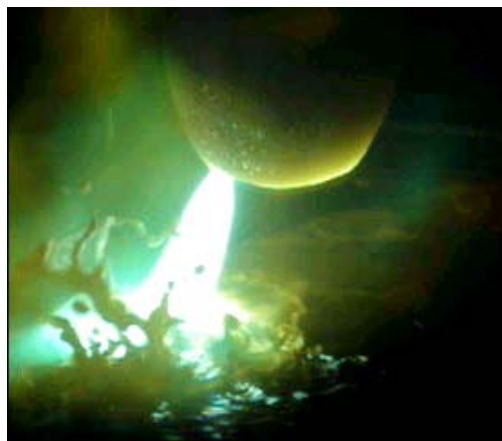
Figure 4.27 Violent splashing at 2 kA (Image L16354)
