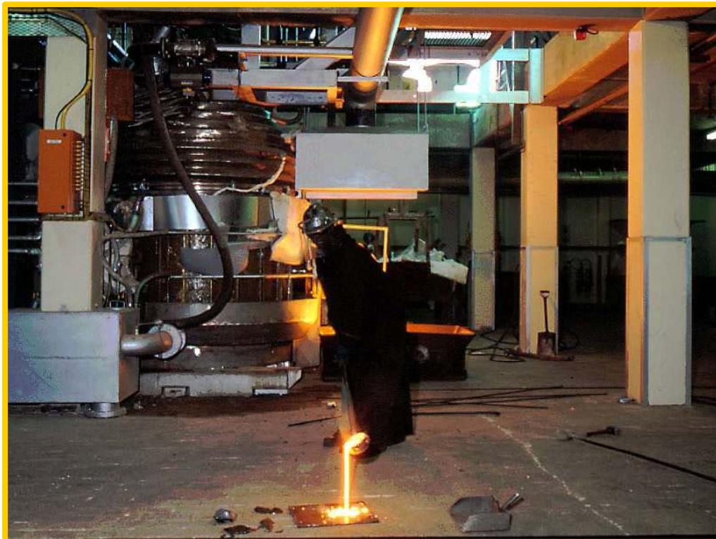
Figure 2.27 Sampling a molten stream from the DC arc furnace for magnesium production
