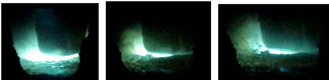
Figure 4.13 Industrial steelmaking arc at 40 kA, 450 V (Full power is at 70 kA, 550 V)
