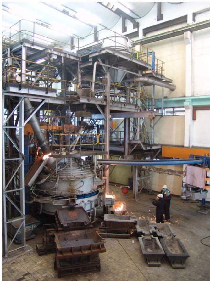
Figure 6.4 Alloy tap from Mintek's 1.5 MW furnace, 2 October 2007
