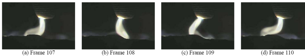
Figure 4.32 Successive frames from a high-speed video sequence showing an arc at 1000 A and 5 cm length, 5000 frames/s, shutter 4 \mu s
