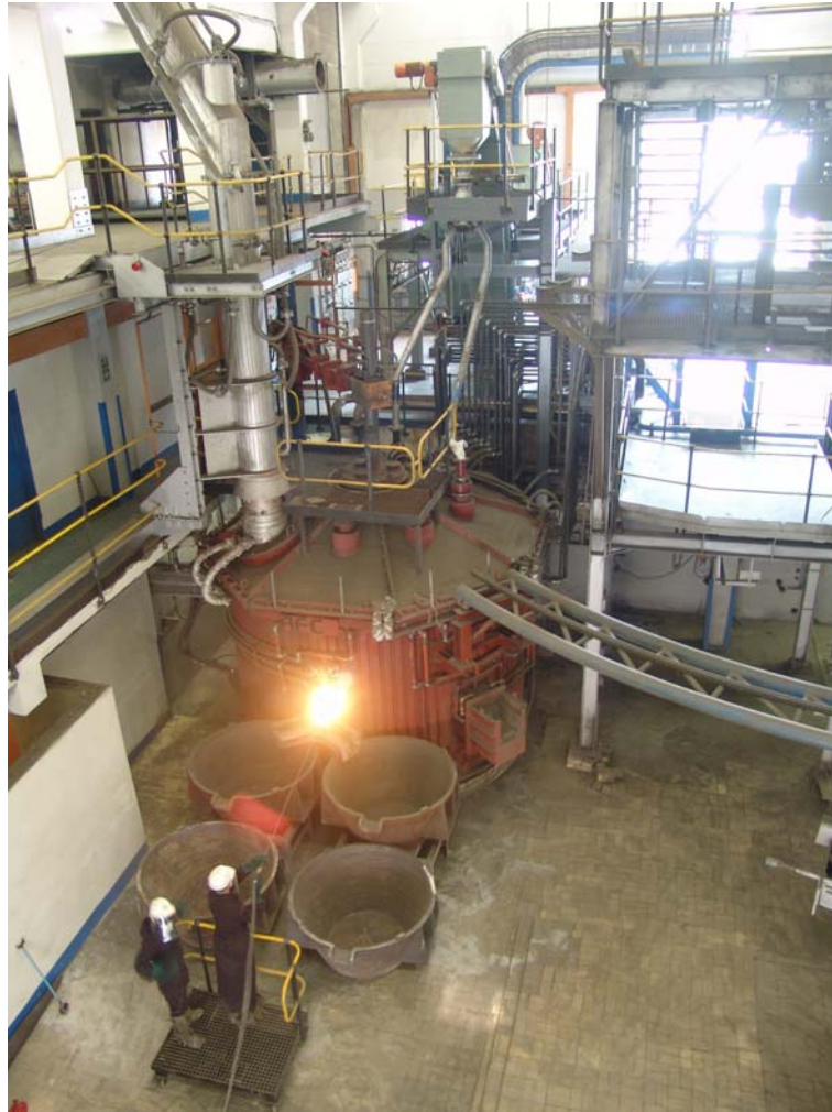
Figure 6.6 First slag tap from Mintek's 3 MW furnace, 4 October 2008
