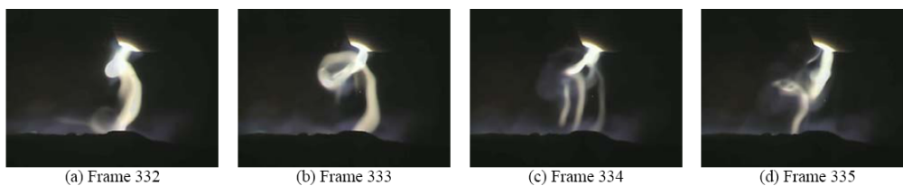
Figure 4.33 Successive frames from a high-speed video sequence showing an arc at 1000 A and 10 cm length, 5000 frames/s, shutter 4 \mu s
