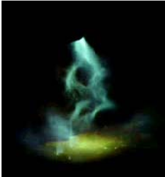
Figure 4.25 'Pretzel-shaped' arc in air on a graphite block
