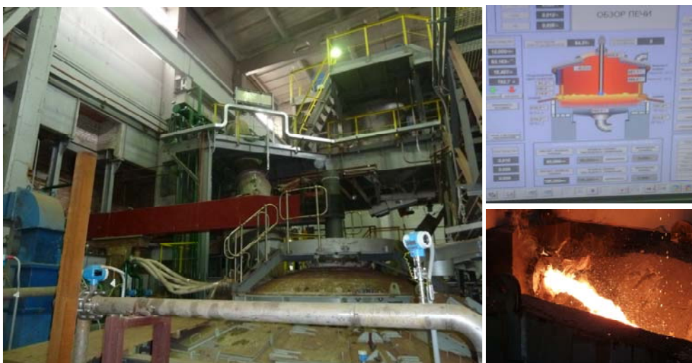
Figure 2.21 A 12 MW DC arc furnace in Orsk, Southern Urals, Russia
