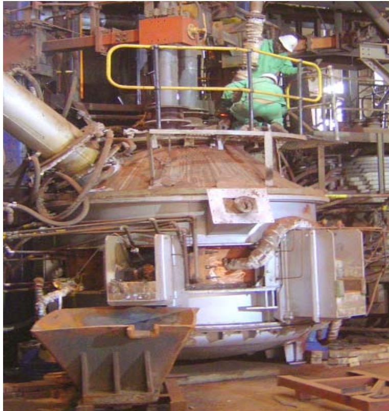
Figure 2.20 A twin-electrode DC arc furnace used for laterite smelting at Mintek
