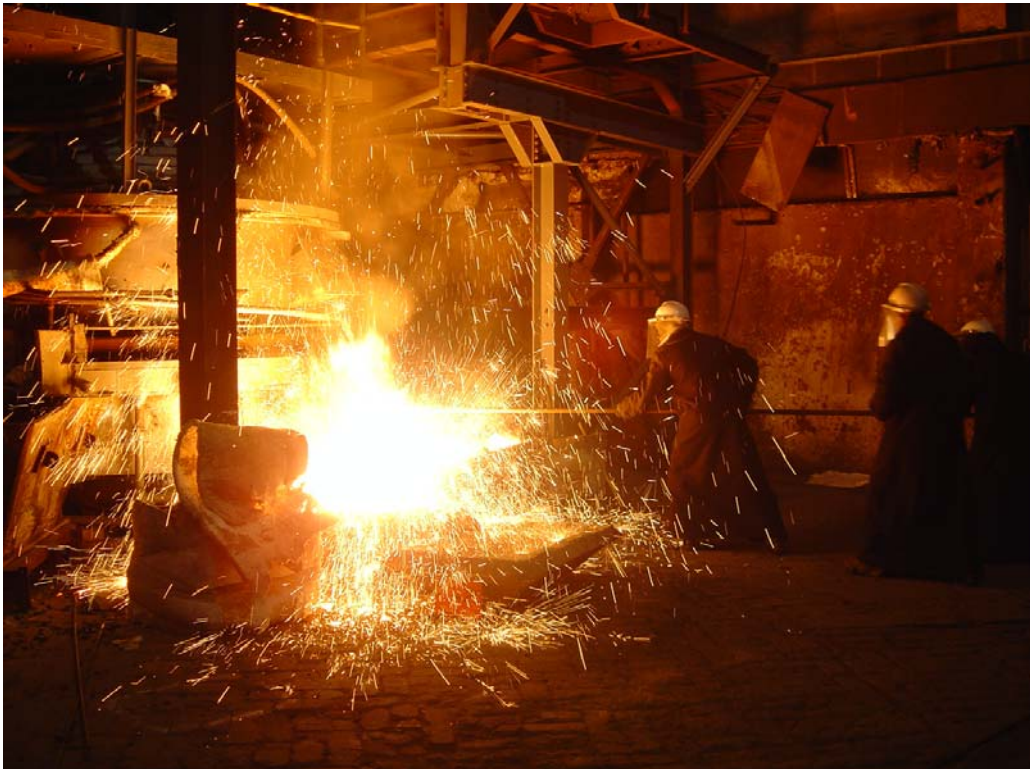
Figure 6.3 Alloy tapping from the 1.5 MW furnace, 16 April 2004 Photograph by Isabel Geldenhuys. Used with permission.
