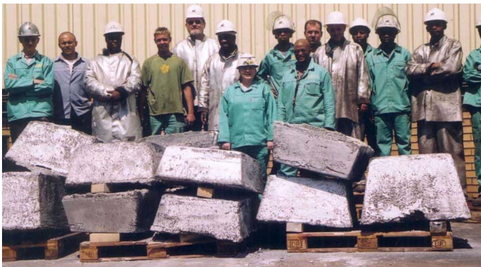
Figure 2.29 Ingots of magnesium produced in a DC arc furnace at Mintek
