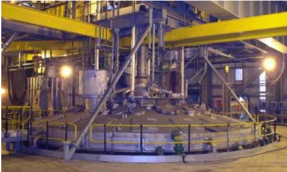
Figure 2.11 Samancor Chrome's first 60 MW furnace in Middelburg
