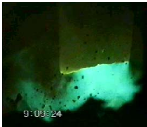
Figure 4.26 Diffuse 7 kA arc onto slag
