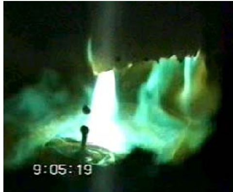
Figure 4.31 Three 'simultaneous' arcs (total current = 2 kA)
