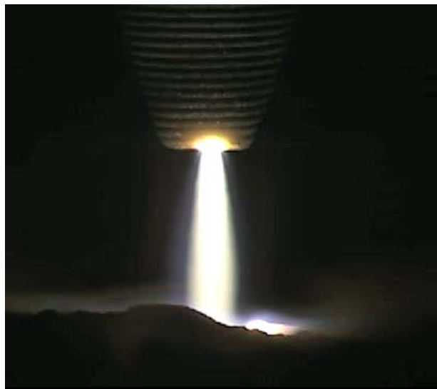
Figure 4.1 Stable arc, 600 A, 5 cm arc length
