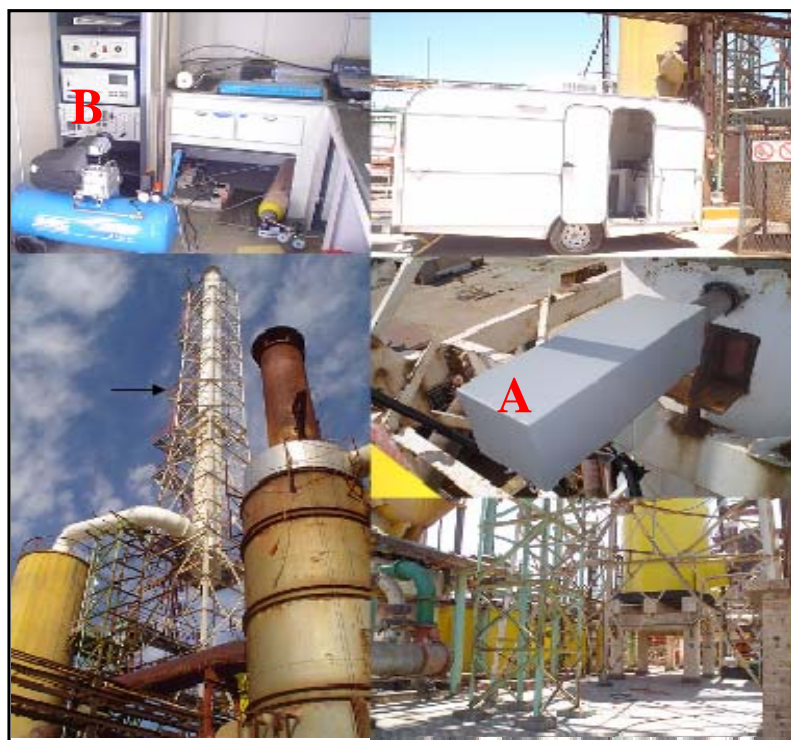
Figure 2.1: The dilution probe that consists of a stack-mounted EPM Sample Probe (A) and SO 2 data analyser (B)
