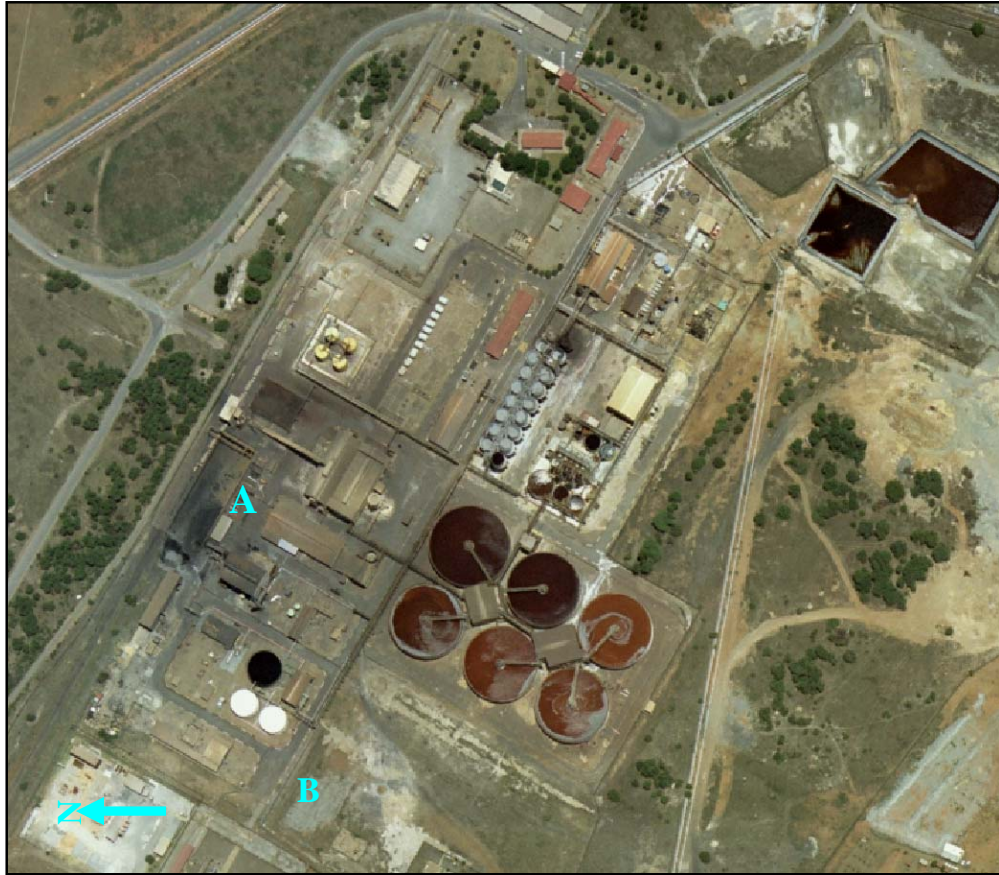
Figure 1.15: South Uranium Plant site. Areas shown in this figure include the six counter current decantation thickeners, boiler stack (A) and the recently commissioned ambient air quality monitoring station (B)
