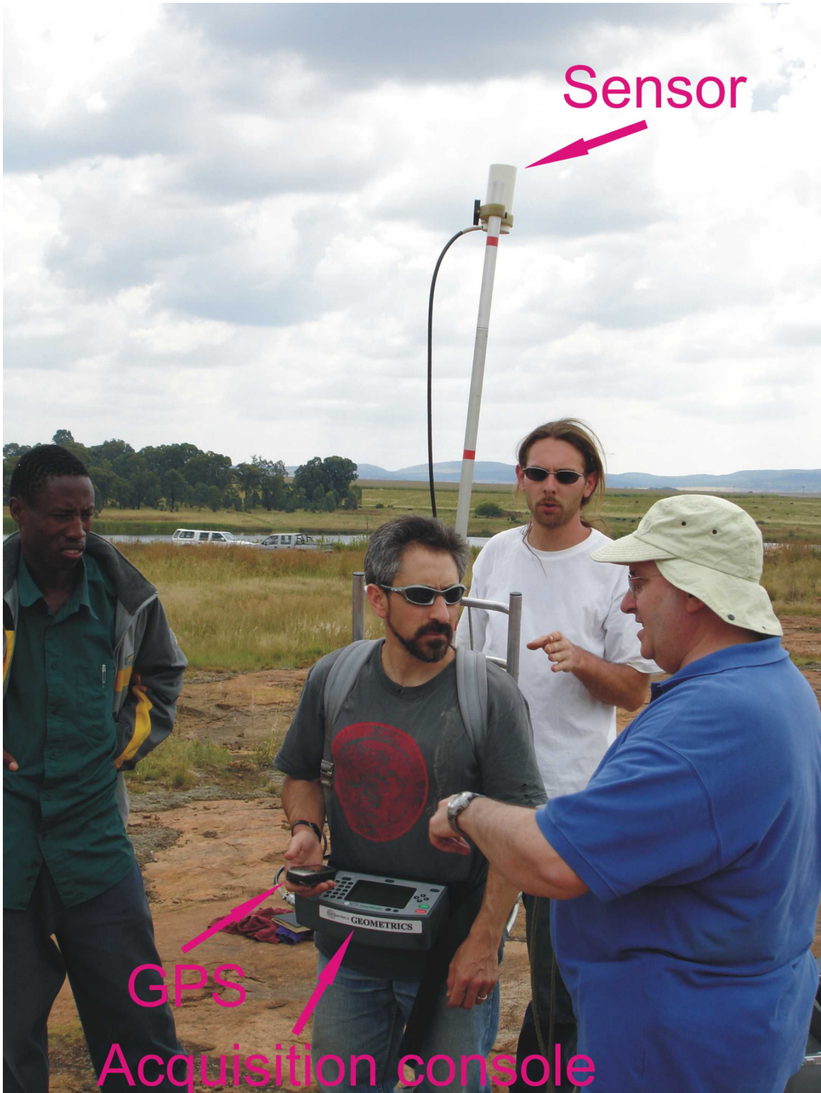
Figure 2.2. Cesium vapour magnetometer, showing the GPS and sensor.
