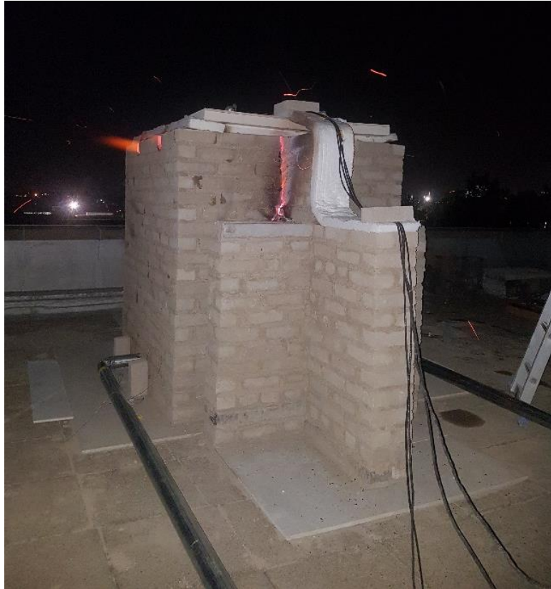
Figure 25. Photograph of lintel test 1 with no load
