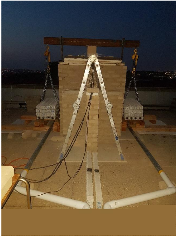
Figure 26. Photograph of lintel test 3 with applied load before ignition
