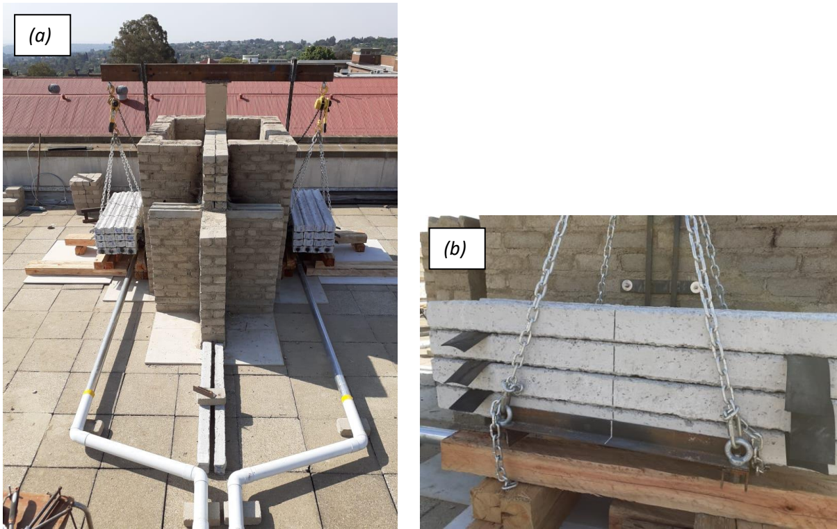
Figure 12. Photographs of (a) furnace loading rig and (b) loading rig weights
