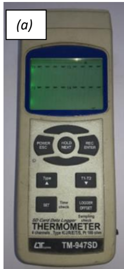
Figure 8. Photograph of (a) Lutron TM947SD 4 channel data logger and (b) type K thermocouple
