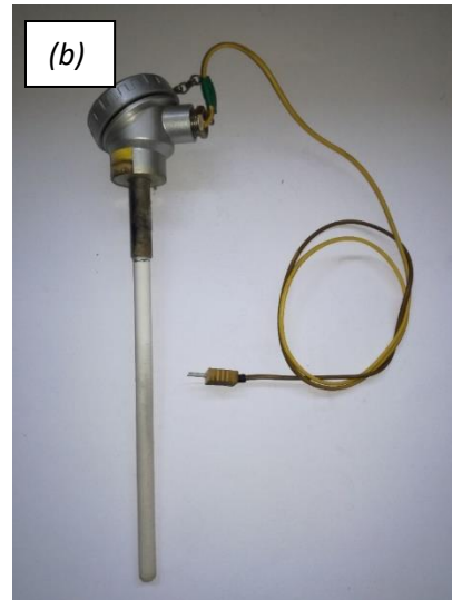
Figure 8. Photograph of (a) Lutron TM947SD 4 channel data logger and (b) type K thermocouple
