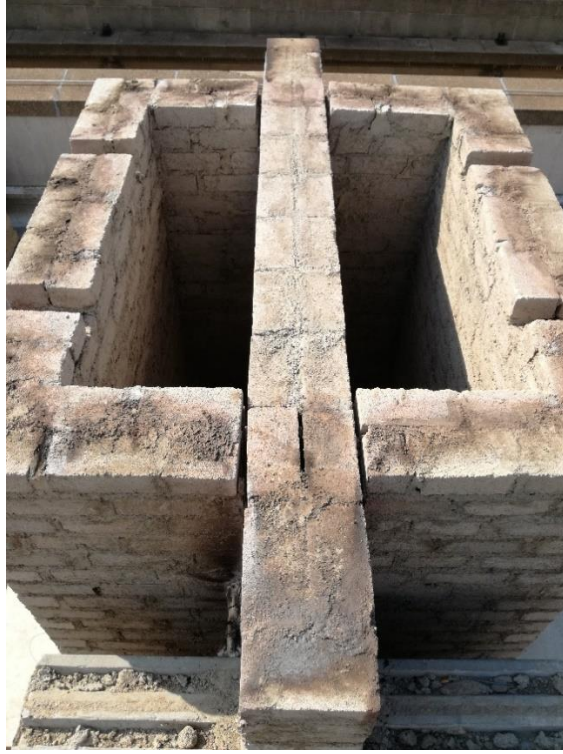
Figure 28. Lintel in furnace approximately 24 hours post test
