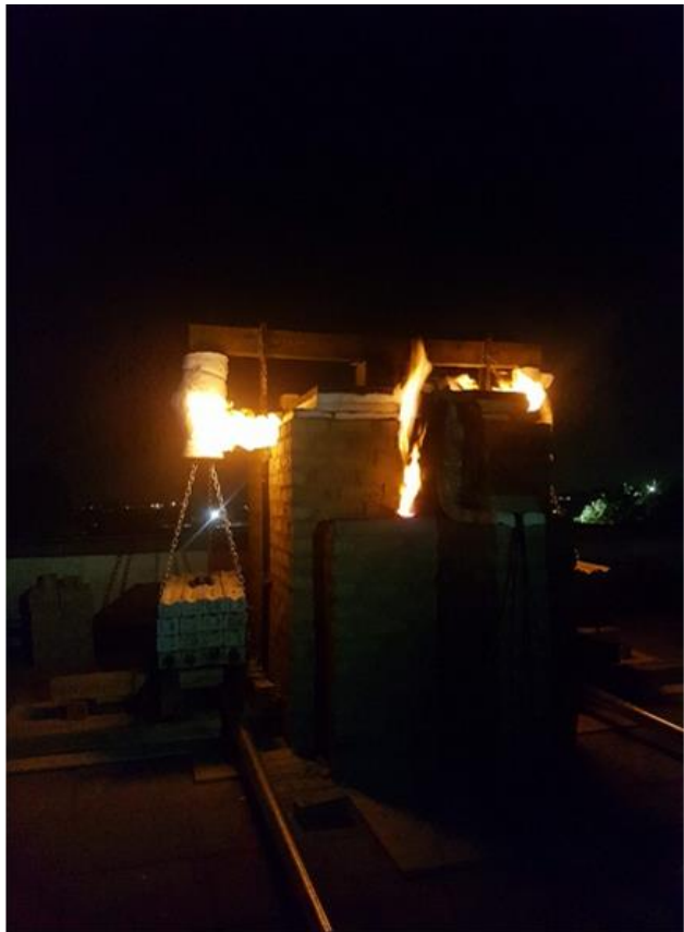
Figure 27. Photograph of lintel test with applied load during fire test
