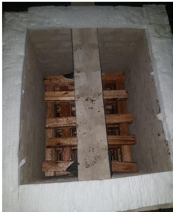
Figure 7. Photograph taken of the timber arrangement inside the furnace
