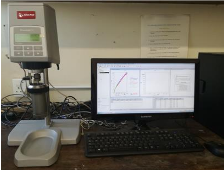
Figure 23: Image of a Rotational rheometer: RheolabQC from Wits - School of Chemical and Metallurgical Engineering. Supplied by Anton Paar, Austria
