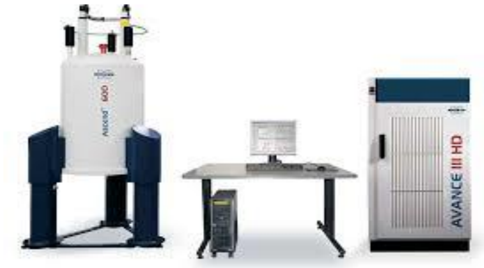
Figure 22: Bruker Ascend 500 Nuclear Magnetic Resonance Spectrometer from University of Johannesburg, Faculty of science. Supplied by Bruker, United States of America.
