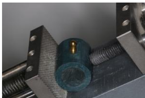
Figure 3.5 Clamped test base with OBZ abutment
