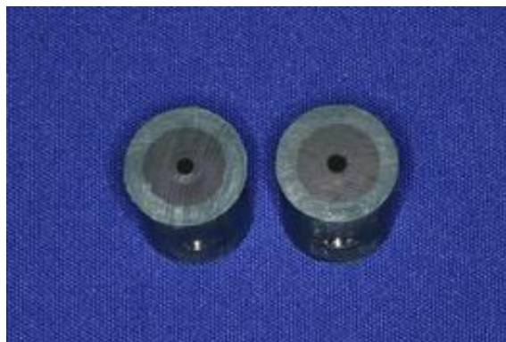
Figure 3.7 Centred holes in test bases containing the metal housings and matrices of both attachment systems
