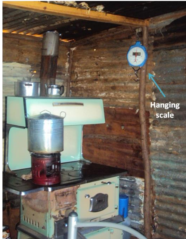
Figure 3.3. Hanging scale set up in a kitchen of one of the 15 study households in Zenzele, used to weigh fuels.
