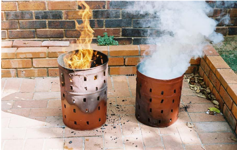
Figure 2.10. The difference between the top-down method and the conventional bottom-up method of lighting a coal fire (Wagner et al. 2005).
