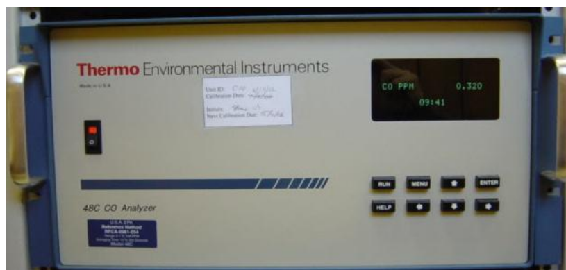
Figure 3.6. TEI 48C CO analyser (APCD, 2003).
