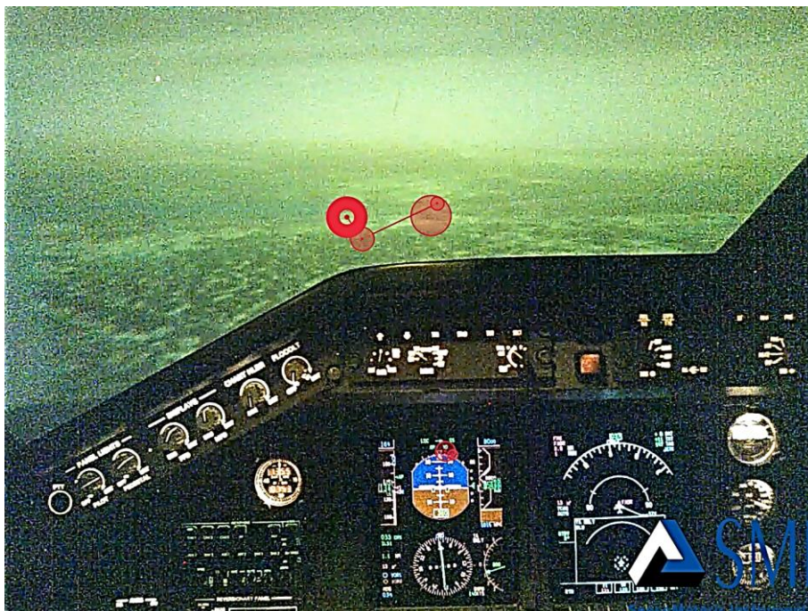
Figure 5-8: Screenshot of visual pattern of pilot during approach on unprepared runway, showing runway. Here the pilot is shown fixating on the runway outside (OUT), with smaller fixations on the virtual horizon (PF) to make sure the aircraft attitude is correct.
