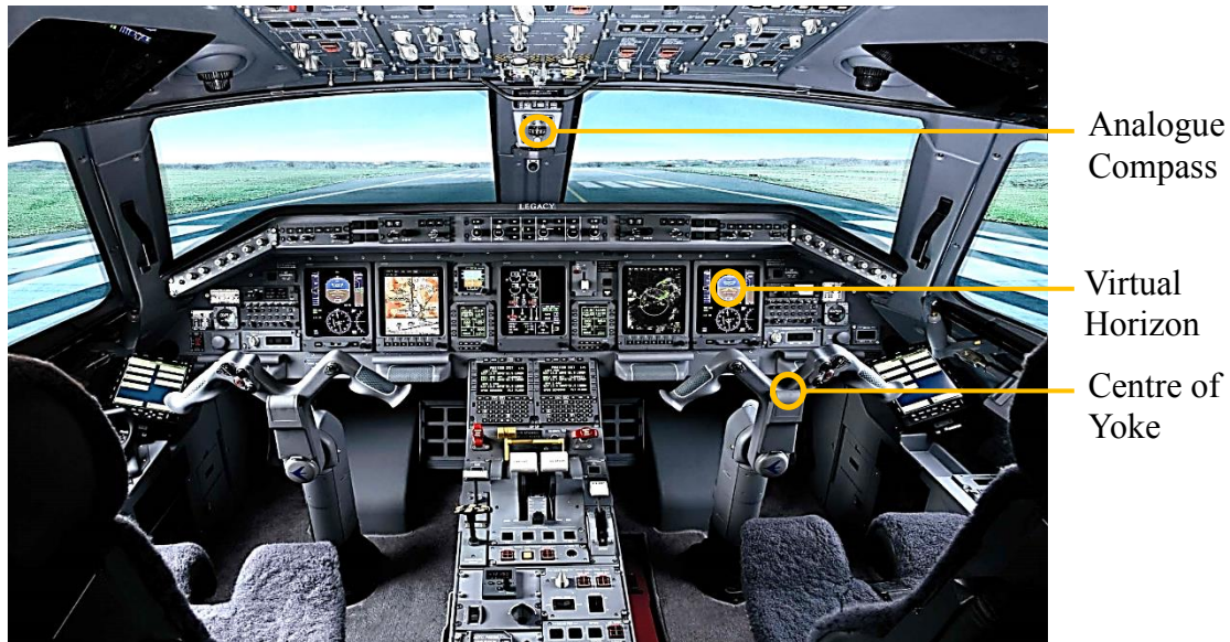
Figure 5-1: Embraer ERJ-145 Simulator, showing calibration points. [44]
