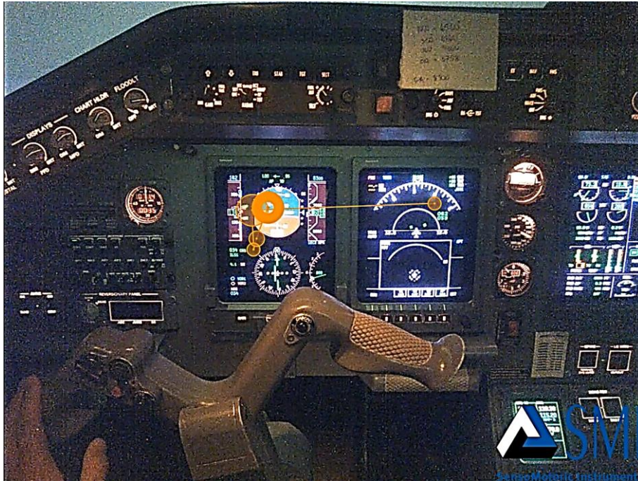
Figure 5-5: Screenshot of visual pattern of pilot during approach on prepared runway. Here the pilot is fixating between the airspeed (PFD), virtual horizon (PFD) and compass heading (ND).
