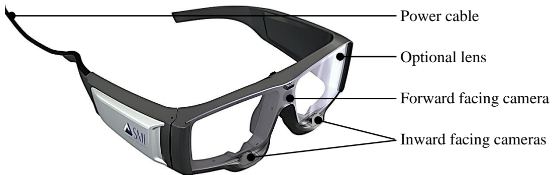
Figure 2-4: SMI Eye Tracking Glasses [16]
