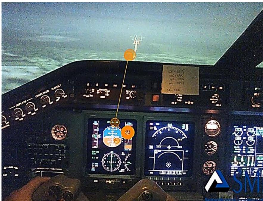
Figure 5-6: Screenshot of visual pattern of pilot during approach on prepared runway, showing runway. Here the pilot is shown fixating between the virtual horizon (PFD), the altitude (PFD) and the runway outside (OUT).
