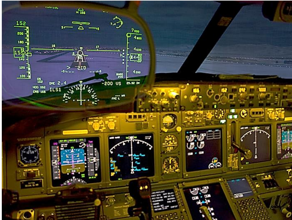
Figure 2-7: Head-up display in a Boeing 737-800 [42].
