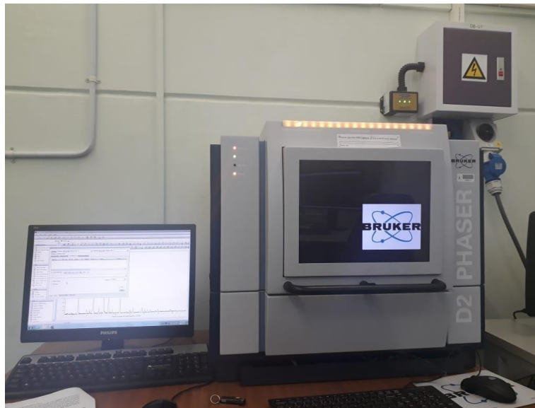
Figure 3.4: Picture of an X-ray diffraction, XRD (model Bruker D2 Phaser) analysis, Wits MMU
