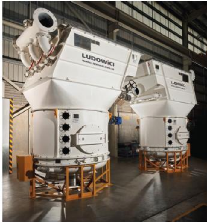
Figure 6.3: RCTM2000 Reflux Classifier (Orupold et al., 2014)
