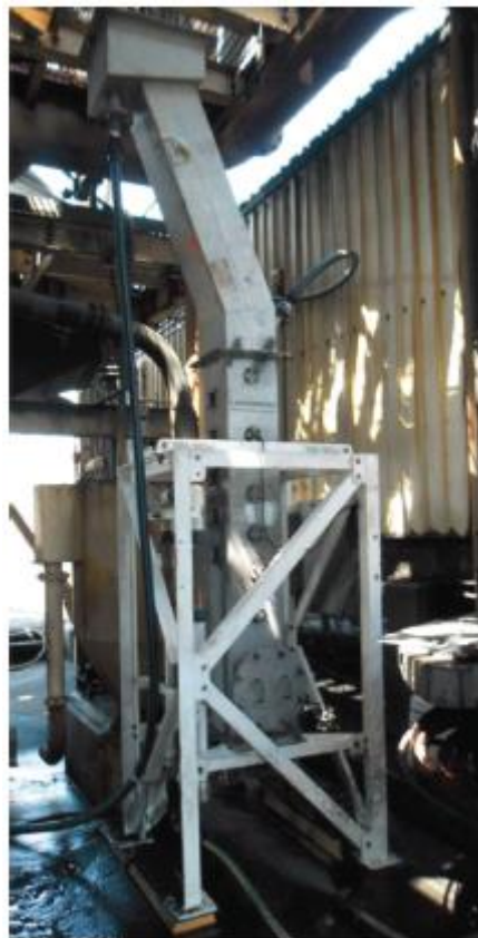
Figure 6.4: RC TM 300 Pilot Scale Reflux Classifier (Orupold et al., 2014)
