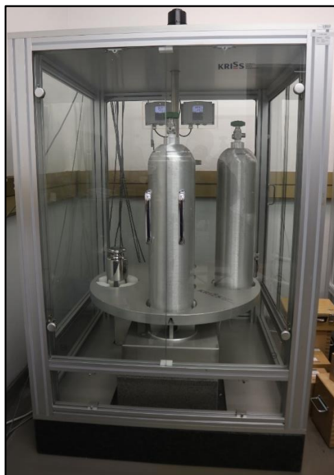
Figure 4.6 A mass comparator with an automated weighing system and a Mettler Toledo balance for weighing gas cylinders.
