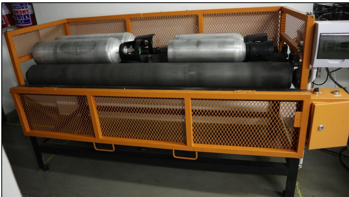
Figure 4.8 Roller bench for the homogenization of gas mixtures.
