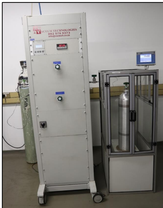
Figure 4.7 Filling station system with a RADWAG mass comparator balance used for gas transfer into the sample cylinder.
