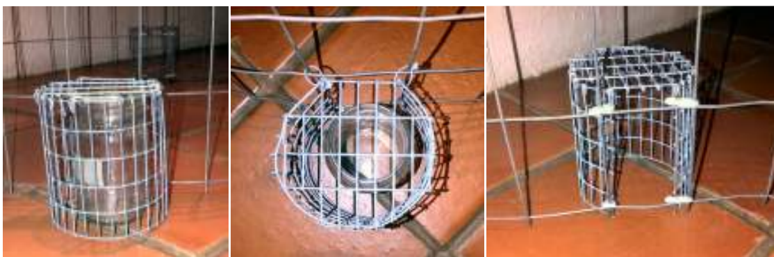
Figure 6. Close up view of holder on a device designed to train scent-matching via proxy in domestic dogs Canis lupus familiaris from front, top and back showing jar placement in holder from front and top angle.
