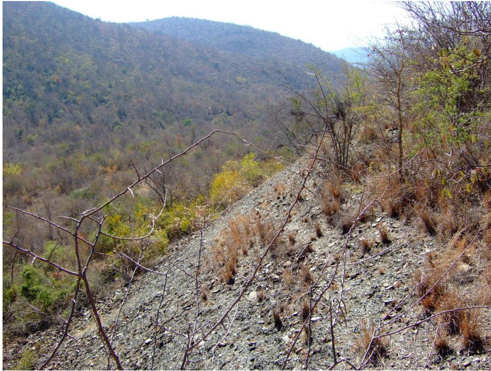
Figure A-3.5: Asbestos waste and fine fibrous material was often end-tipped at steep elevations just outside shaft entrances (Source: Author)
