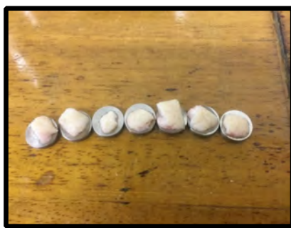
Figure 7.5: Illustration of porcine skin divided into 4-5 mm sections to be mounted in flow-through diffusion cells (exposed area 0.039 cm 2 ).
