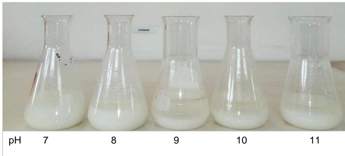
Figure 4.7: Waste water treated with \text{MgCl}_2\cdot 6\text{H}_2\text{O} and 85% \text{H}_3\text{PO}_4 , pH, 7, 8, 9, 10 and 11 adjusted with 10% KOH, at 25°C
