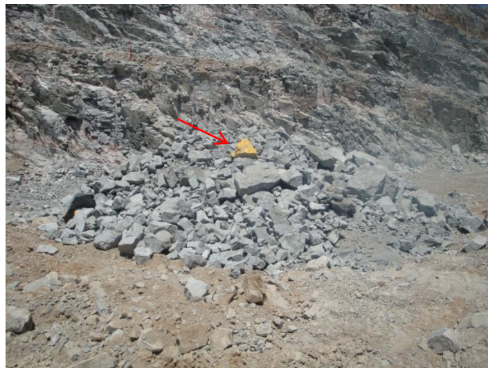
Figure 3-3: A muck pile showing one of the blocks selected for rock-fall testing.
