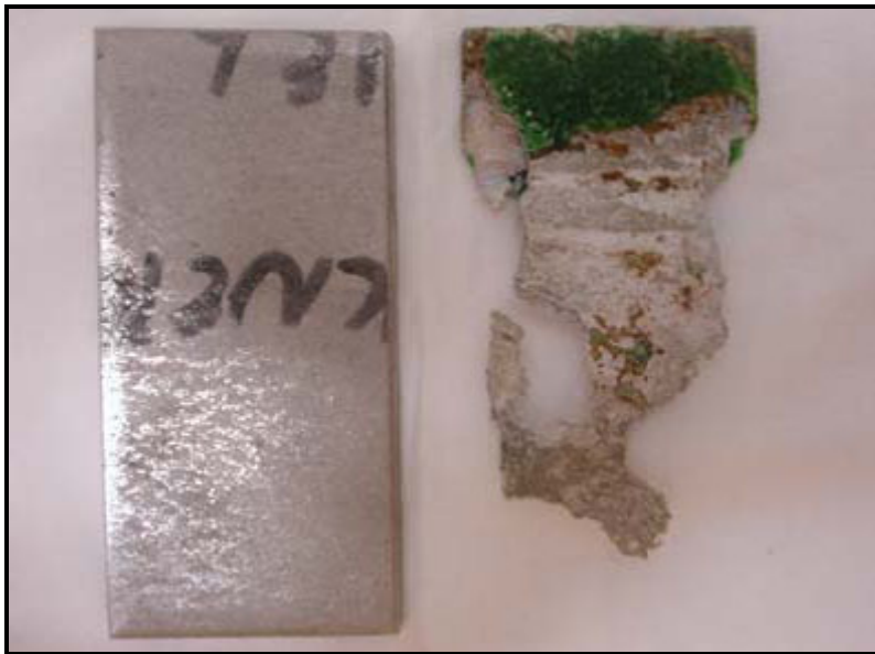
Figure 9: Condition of stainless steel before and after testing. Photograph sourced from Osborne et al., 2002.
