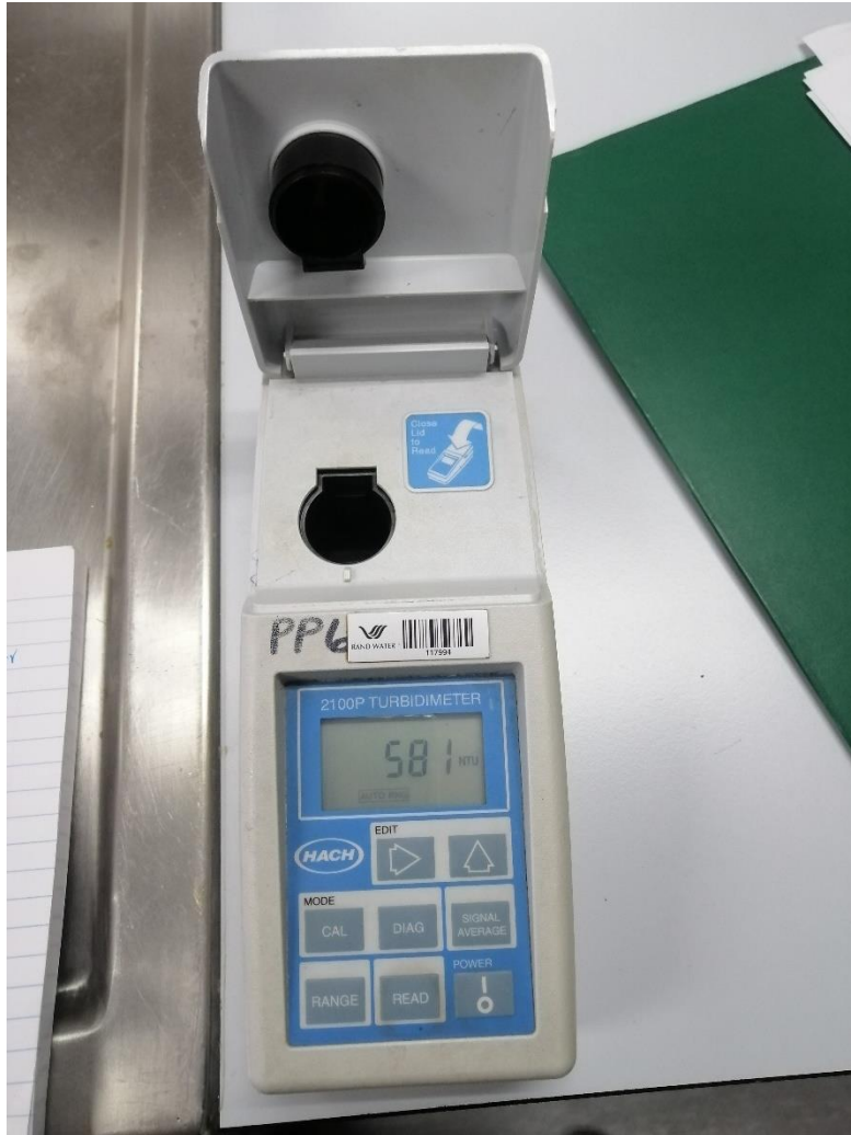
Figure A1. 2: The turbidity meter used to measure initial and residual turbidity.
