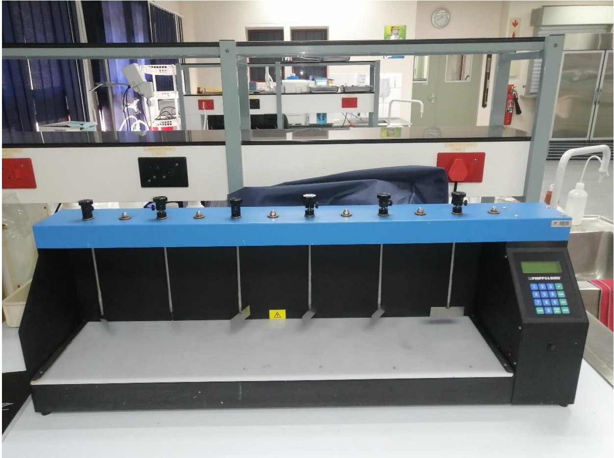
Figure A1. 1: The Jar Test apparatus used for coagulation and flocculation processes.
