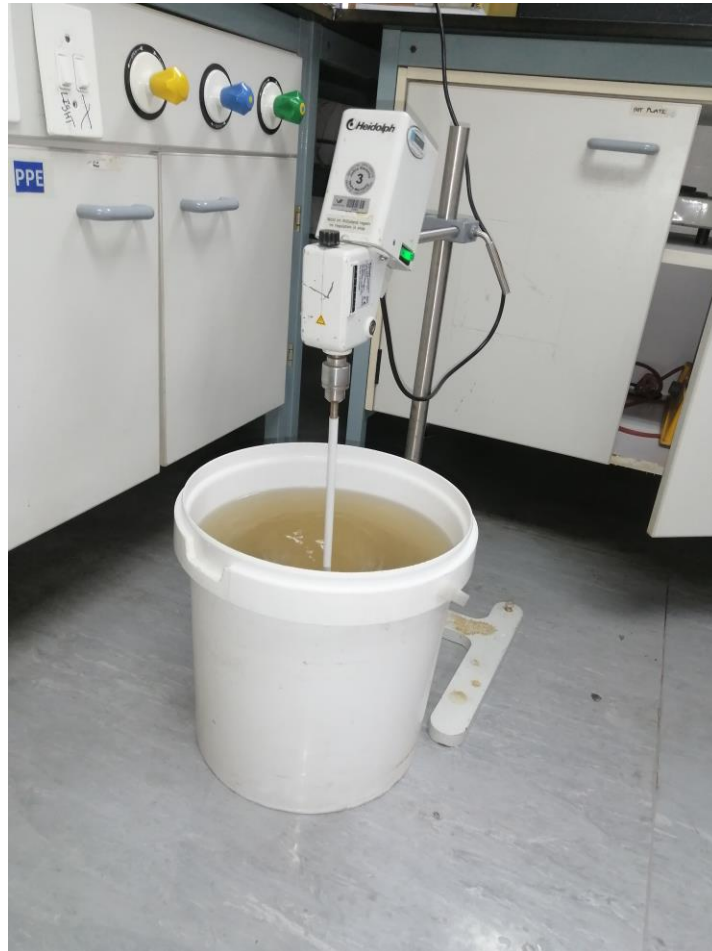
Figure 3. 3 : The Vaal Water feed water preparation.
