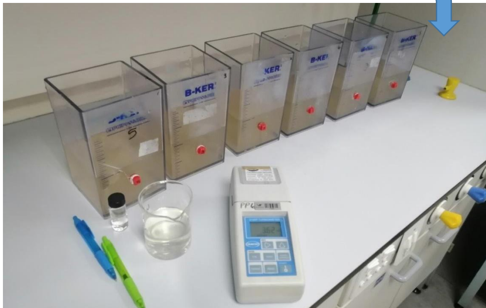
Figure 3. 7: Initial and Residual Turbidity Measurement with a turbidity meter.
