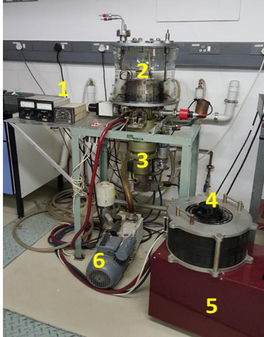
Figure 3.6: A photograph of thermal evaporation setup showing the following: (1) Penning gauges, (2) vacuum chamber, (3) diffusion pump, (4) variac, (5) power supply and (6) rotary pump.
