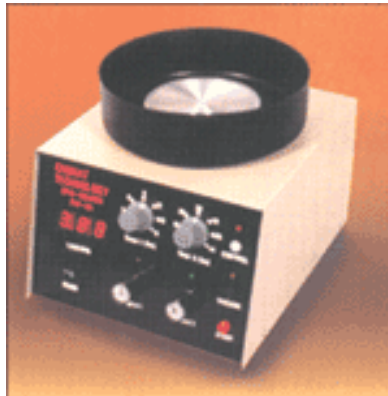
Figure 3.4: A photograph of the 2-stage CHEMAT precision spin coater.
