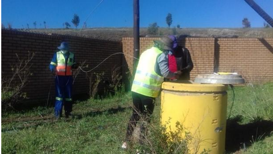
Figure 4-1: Measuring physicochemical parameters in the Marie Louise landfill site
