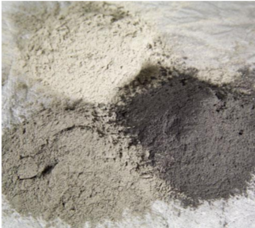
Figure 2.3: Typical colours of coal fly ash (ACAA, 2015).
