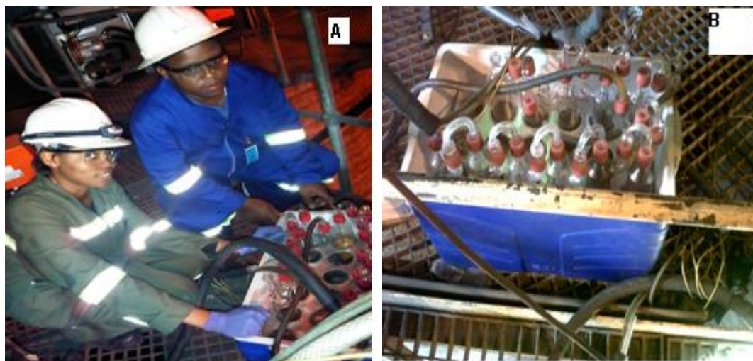
Figure 6.2: Sampling at the stack in Duvha Power Station: (A) Sampling personnel; (B) Sampling train.
