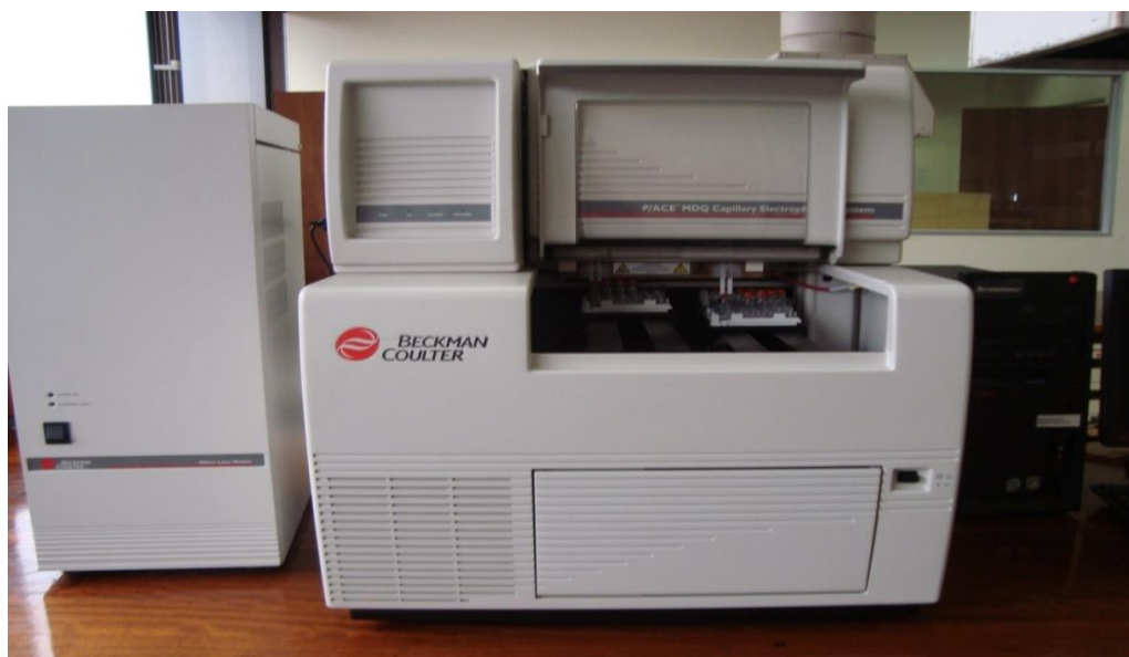
Figure A2.1: Beckman Coulter P/ACE MDQ instrument for capillary electrophoresis.
