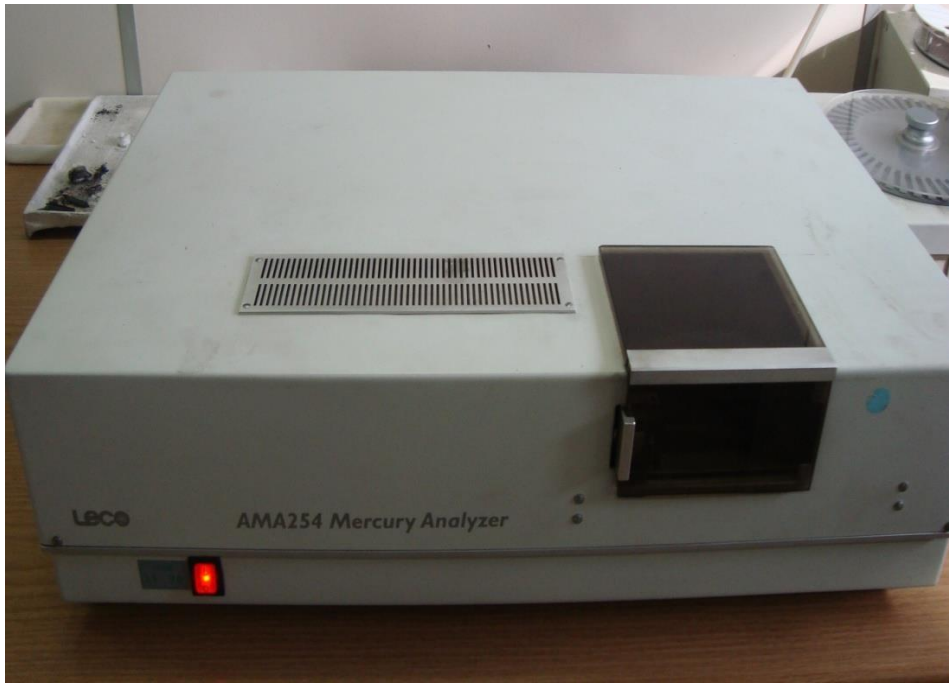
Figure A2.3: Leco AMA 254 mercury analyzer for direct Hg analysis.
