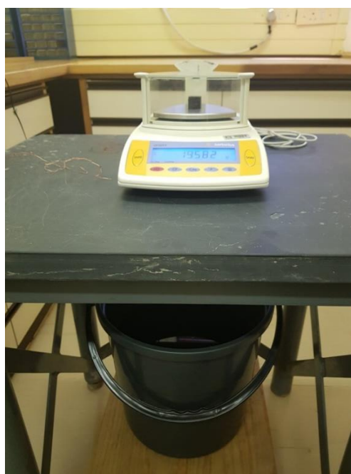
Figure 6-6 Sartorius equipment used for density measurements. The bucket contains water to immerse the suspended sample with a copper wire.
