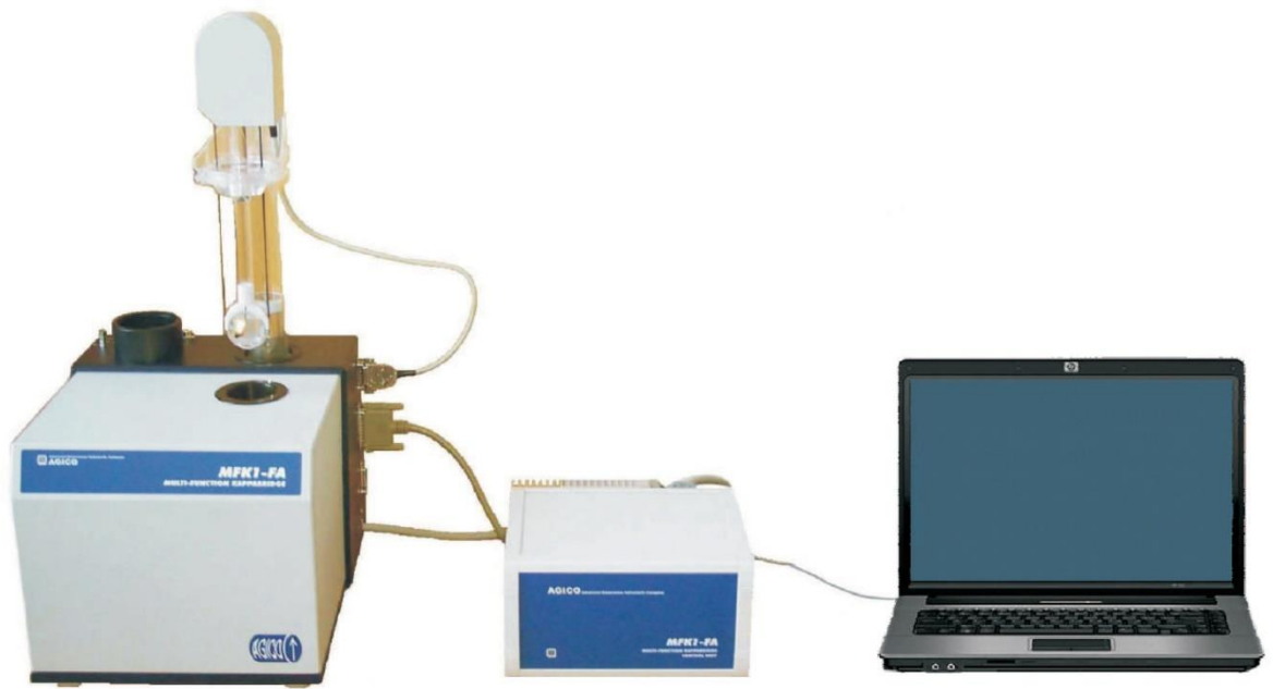
Figure 6-2 MFK1-FA multi-function kappabridge instrument setup was used to measure bulk magnetic susceptibility (AGICO).
