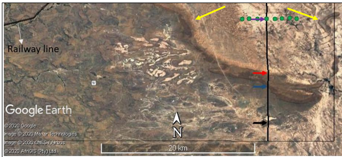
Figure 8-8 Anomaly 4 location (purple arrow) on Google Earth image with seismic profile BV21 marked (black line) and MT stations (green markers). The anomaly could be due to a buried inclined sheet linking the outcropping sheet to the west and east (shown by yellow arrows).
