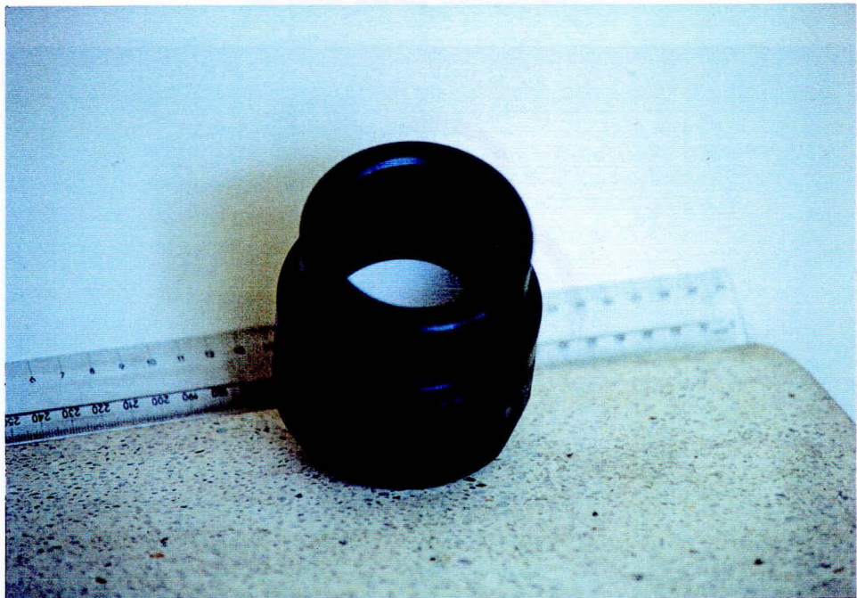
Fig.9.4. A cylindrical section threaded into the base segment, pressing the O-ring tight against the filter.
