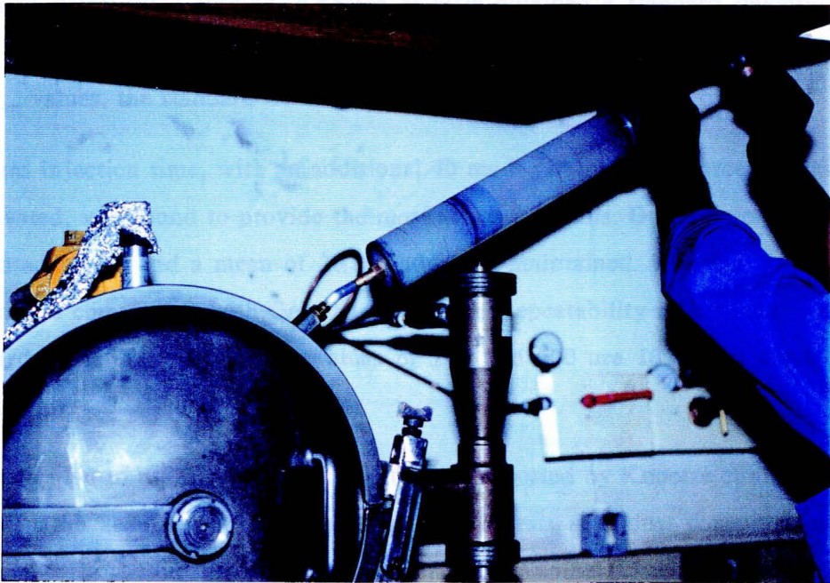
Fig.6.16. Methane addition to the explosion vessel.
