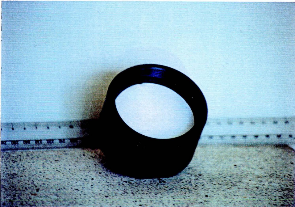
Fig.9.2. The filter laid into position in the base segment of the sampling pot.
