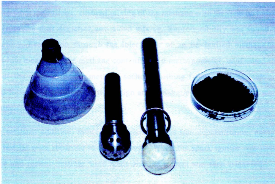
Fig.6.15. The "pepperpot" dust sample holder.
