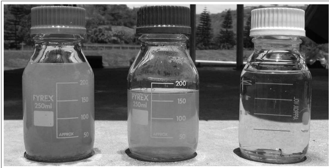
Figure A.11: Three sample bottles, from left to right - ABR influent, ABR effluent and membrane filtrate.
