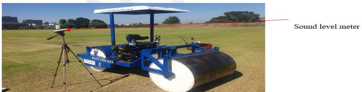
Figure 3: SLM mounted on a tripod stand with the microphone pointing towards the source
